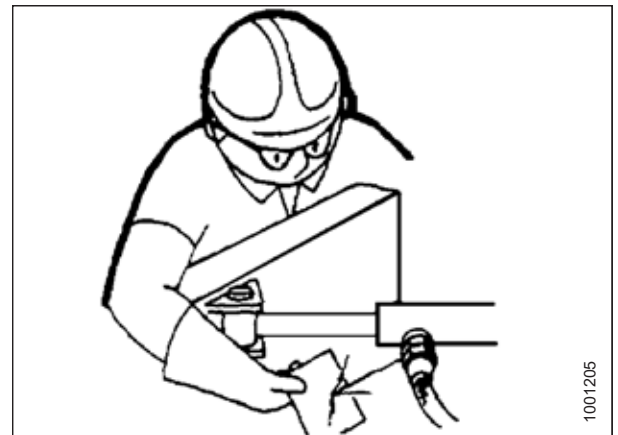
Figure 4.279: Test de fuites hydrauliques
