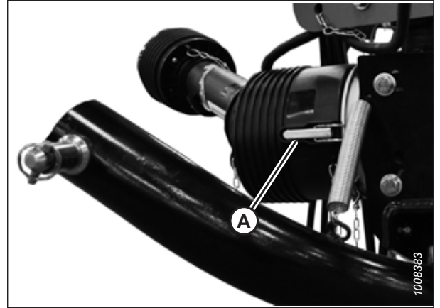
Figure 4.189: Shield Clipped to Driveline
