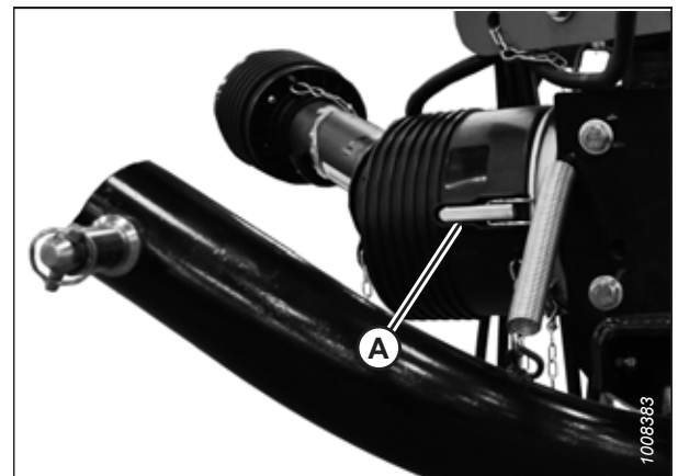
Figure 4.185: Driveline Shield Cone and Lever Clamp
