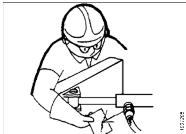
Figure 1.8: Testing for Hydraulic Leaks
