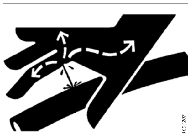
Figure 1.9: Hydraulic Pressure Hazard
