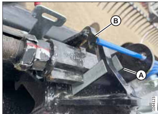
Figure 6.47: Installation de la cale
