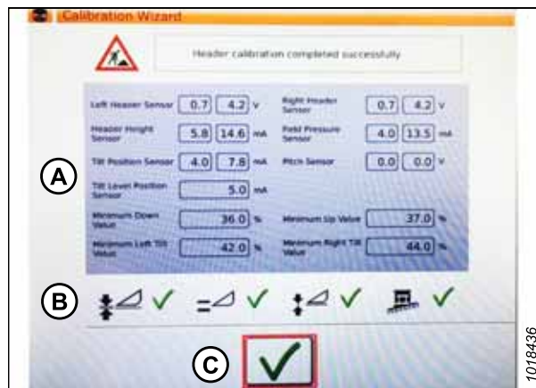
Figure 3.650: Completed Calibration Page
