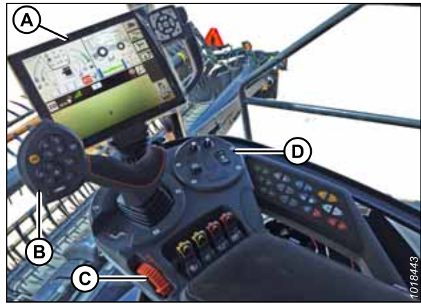
Figure 3.622: Operator’s Station – Gleaner® S9 A - Tyton Terminal B - Control Handle C - Throttle D - Header Control Cluster
