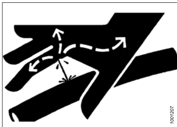
Figure 1.12: Hydraulic Pressure Hazard
