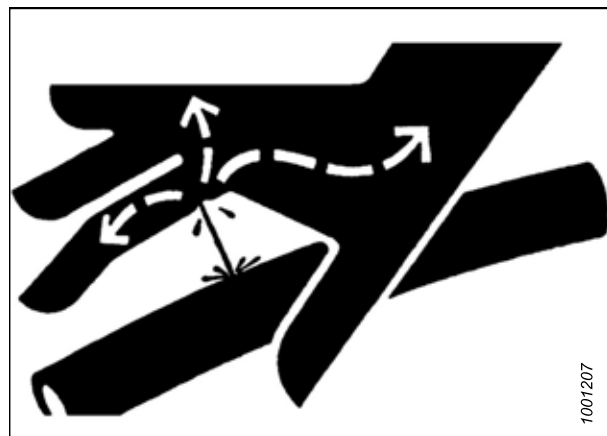
Figure 4.1: Hydraulic Pressure Hazard
