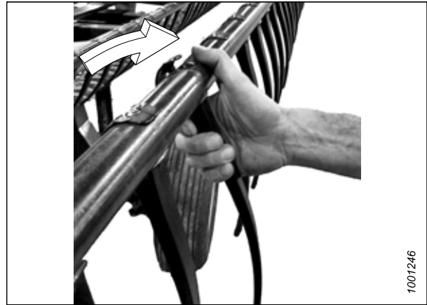
Figure 4.281: Installing Plastic Finger
