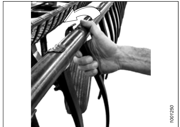
Figure 4.280: Removing Plastic Finger
