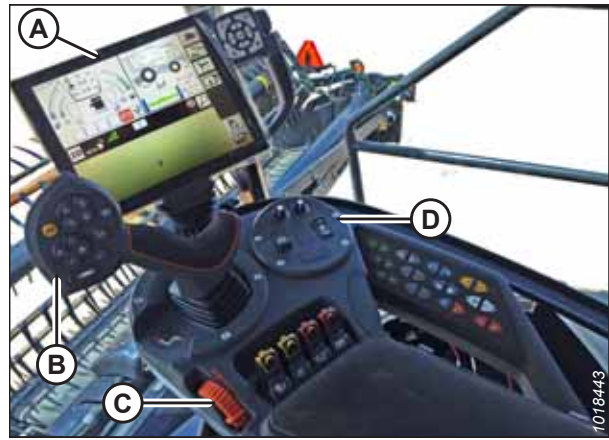
Figure 8.196: Operator’s Station – Gleaner® S9 A - Tyton Terminal B - Control Handle C - Throttle D - Header Control Cluster
