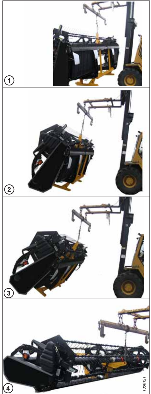
Figure 2.18: Lowering Header to the Ground
