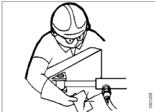
Figure 1.8: Testing for Hydraulic Leaks
