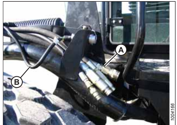
Figure 3.41: Header Drive Hoses
