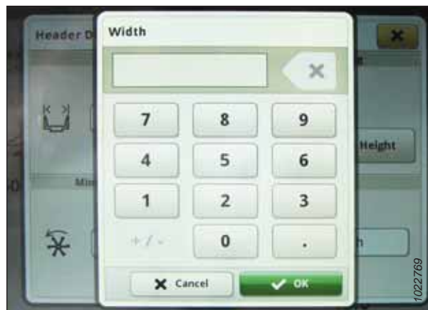
Figure 3.741: John Deere S7 ekraan – heedri laiuse seadistamine
