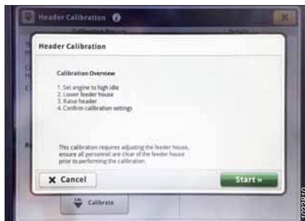
Figure 3.766: John Deere S7 ekraan – heedri kalibreerimine
