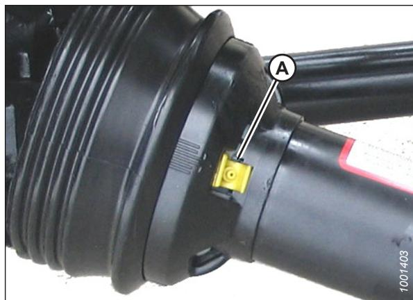
Figure 4.58: Protection de transmission
