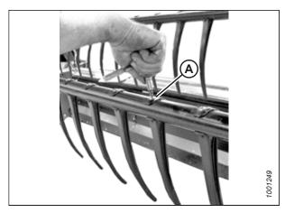
Figure 4.298: Installing Plastic Finger
