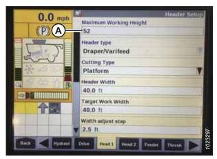
Figure 3.278: Case Combine Display – Header Setup Page
