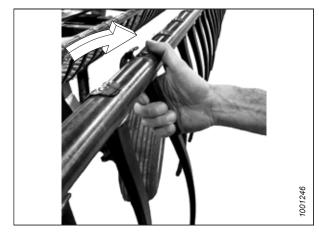
Figure 4.297: Installing Plastic Finger
