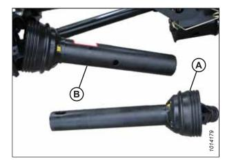
Figure 4.52: Separated Driveline
