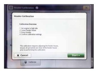
Figure 3.766: John Deere S7 Display – Header Calibration
