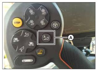
Figure 3.671: AHHC on Control Handle
