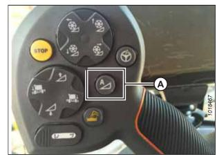
Figure 3.640: AHHC on Control Handle
