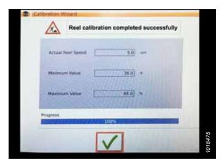
Figure 3.624: Calibration Progress
