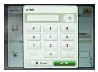
Figure 3.741: John Deere S7 Display – Setting Header Width
