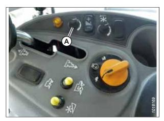
Figure 3.513: Height Adjustment Knob on the Combine Control Console
