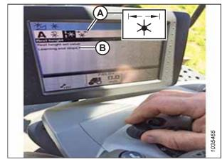
Figure 3.567: CLAAS Combine Display and Console
