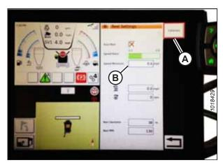
Figure 3.622: Reel Settings Calibration
