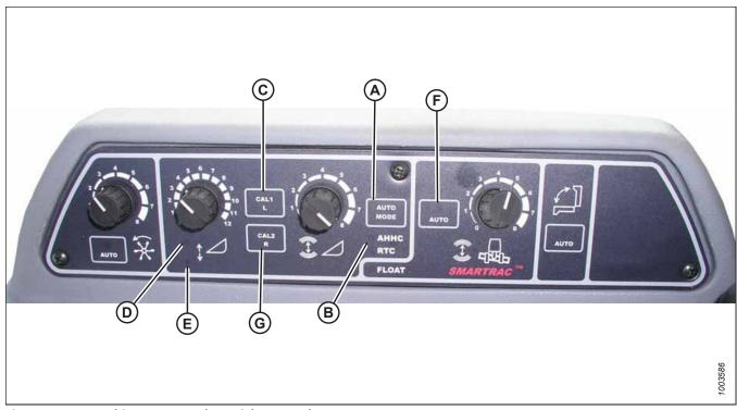
Figure 3.602: Combine Auto Header Height Controls
