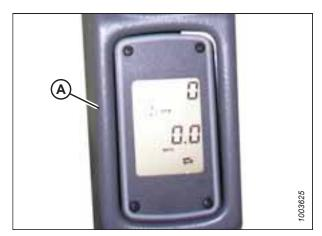
Figure 3.608: Tachometer
