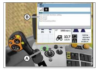
Figure 3.558: CLAAS Combine Display, Console, and Control Handle
