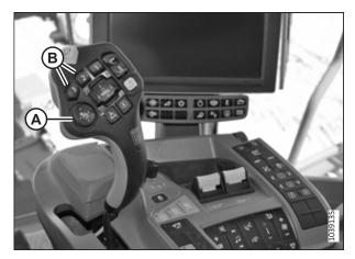
Figure 3.787: John Deere X9 - Multi-Function Lever
