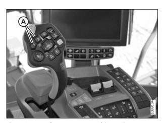
Figure 3.786: John Deere X9 – Multi-Function Lever
