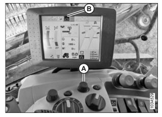
Figure 3.49: Draper Speed Icon on Older CLAAS Machines
