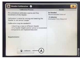
Figure 3.764: John Deere S7 Display – Header Calibration
