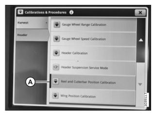
Figure 3.778: John Deere X9 Display – Reel and Cutterbar Position Calibration
