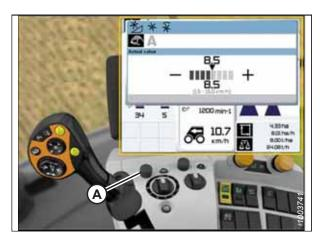
Figure 3.560: CLAAS Combine Display, Console, and Control Handle
