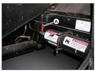
Figure 3.603: Combine Accumulator ON/OFF Switch
