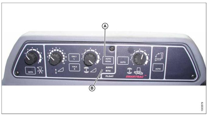
Figure 3.600: Combine Auto Header Height Controls
