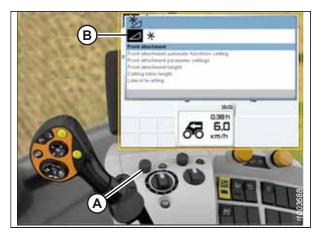
Figure 3.547: CLAAS Combine Display, Console, and Control Handle
