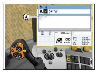
Figure 3.559: CLAAS Combine Display, Console, and Control Handle
