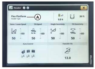
Figure 3.739: John Deere S7 Display - Header Page
