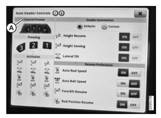
Figure 3.785: John Deere X9 Display – Auto Header Controls Page
