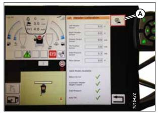
Figure 3.633: Header Calibration
