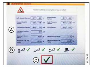
Figure 3.636: Completed Calibration Page
