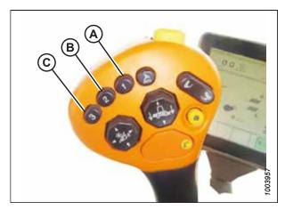
Figure 3.716: Control Handle Buttons
