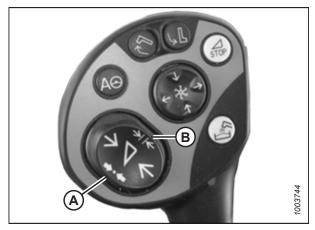
Figure 3.530: Control Handle Buttons
