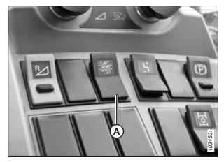
Figure 3.261: Header Function Switch
