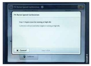
Figure 3.759: John Deere S7 Display – Feeder House Calibration
