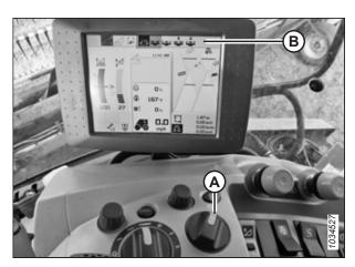
Figure 3.47: Hot Key Position for Draper Speed Control
