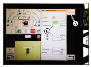
Figure 3.657: Reel Settings Calibration
