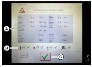
Figure 3.667: Completed Calibration Page
