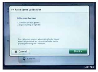
Figure 3.758: John Deere S7 Display – Feeder House Calibration
