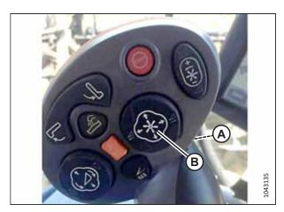
Figure 3.260: Multifunction Handle - New Holland
