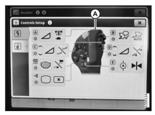
Figure 3.57: John Deere X9 Display – Controls Setup
