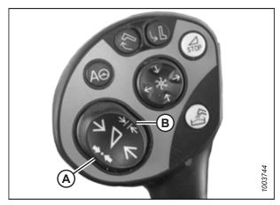
Figure 3.542: CLAAS Control Handle Buttons
