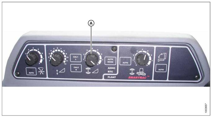
Figure 3.607: Auto Header Height Control Console
