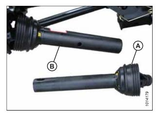
Figure 4.52: Separated Driveline
