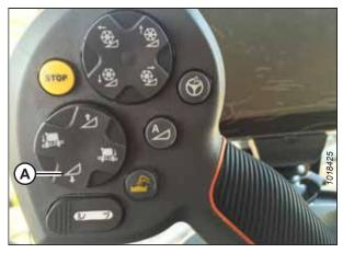
Figure 3.632: Header Down Switch
