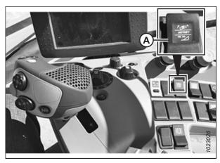
Figure 3.266: Multifunction Lever Toggle Switch
