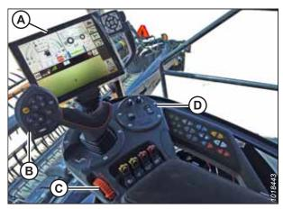
Figure 3.610: Operator's Station - Gleaner S9°
