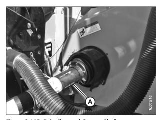
Figure 3.115: Driveline and Output Shaft
