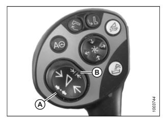
Figure 3.538: CLAAS Control Handle Buttons
