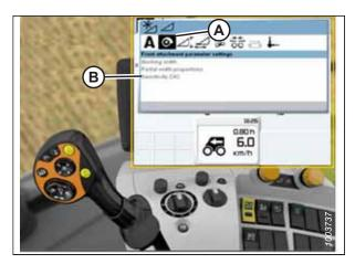
Figure 3.555: CLAAS Combine Display, Console, and Control Handle
