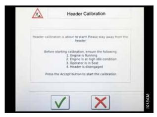
Figure 3.634: Header Calibration Warning
