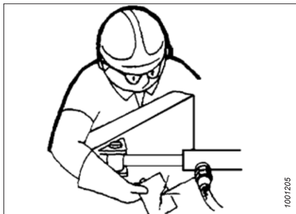
Figur 5.2: Test for hydrauliklækager
