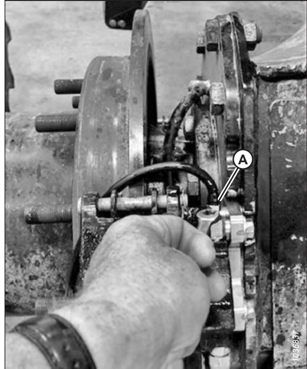
Figure 4.31: Drain Hose Attached to Bleed Screw
