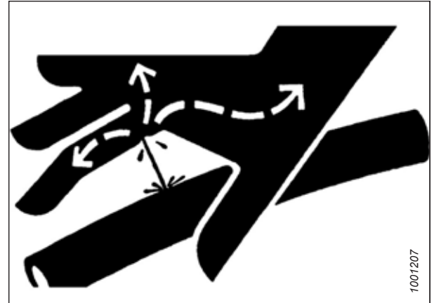
Figure 5.5: Hydraulic Pressure Hazard
