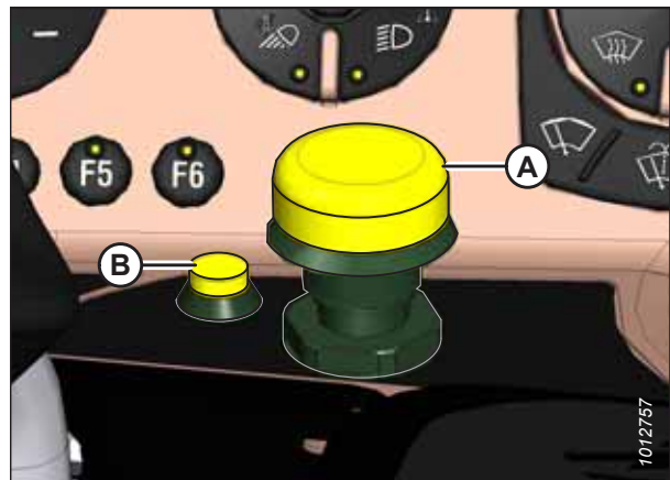
Figure 3.58: Header Drive Controls
