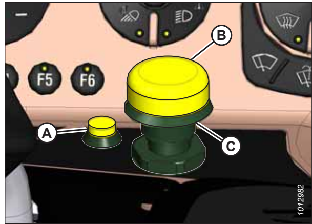
Figure 5.107: Header Drive Controls
