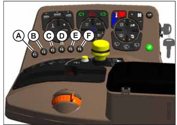
Figure 3.56: Operator's Console Shortcut Buttons
