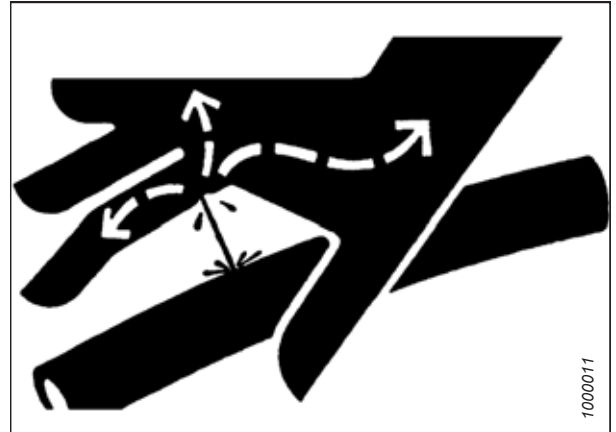
Figure 6.27: Hydraulic Pressure Hazard
