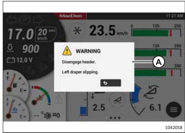
Figure 5.144: Draper Slip Warning
