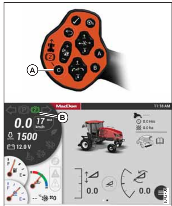
Figure 3.67: Secondary Braking System Button on GSL
