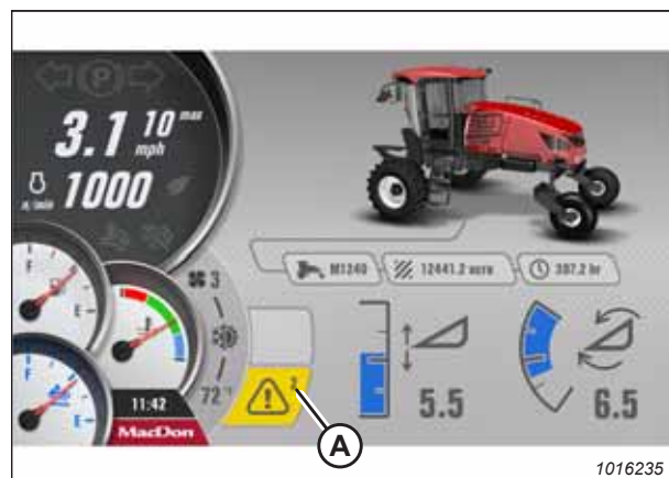
Figure 3.136: Telltale Icon – Multiple Faults Detected
