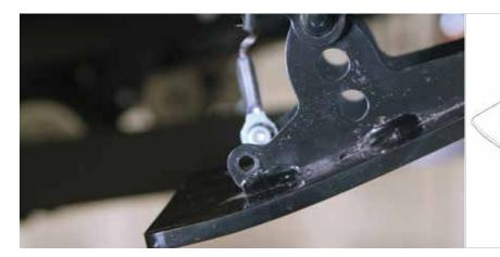
WHAT IT DOES The High Wear Skid Shoes kit provides extended wear skid shoes for use in rocky, abrasive conditions.
