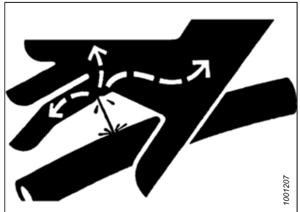
Figure 1.9: Hydraulic Pressure Hazard
