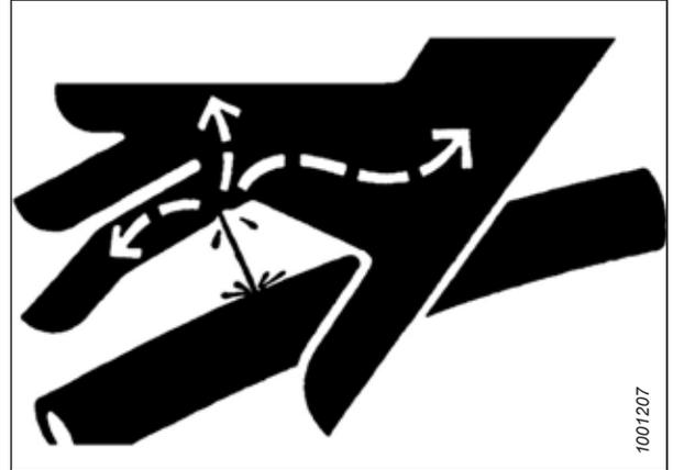
Figure 5.1: Hydraulic Pressure Hazard
