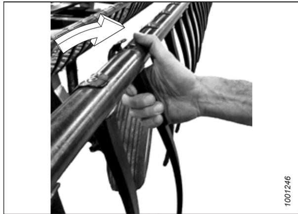
Figure 5.138: Installing Plastic Finger
