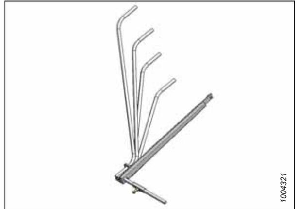
Figure 6.8: Swath Forming Rods
