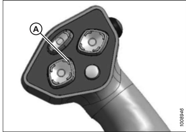
Figure 4.59: Ground Speed Lever (GSL)
