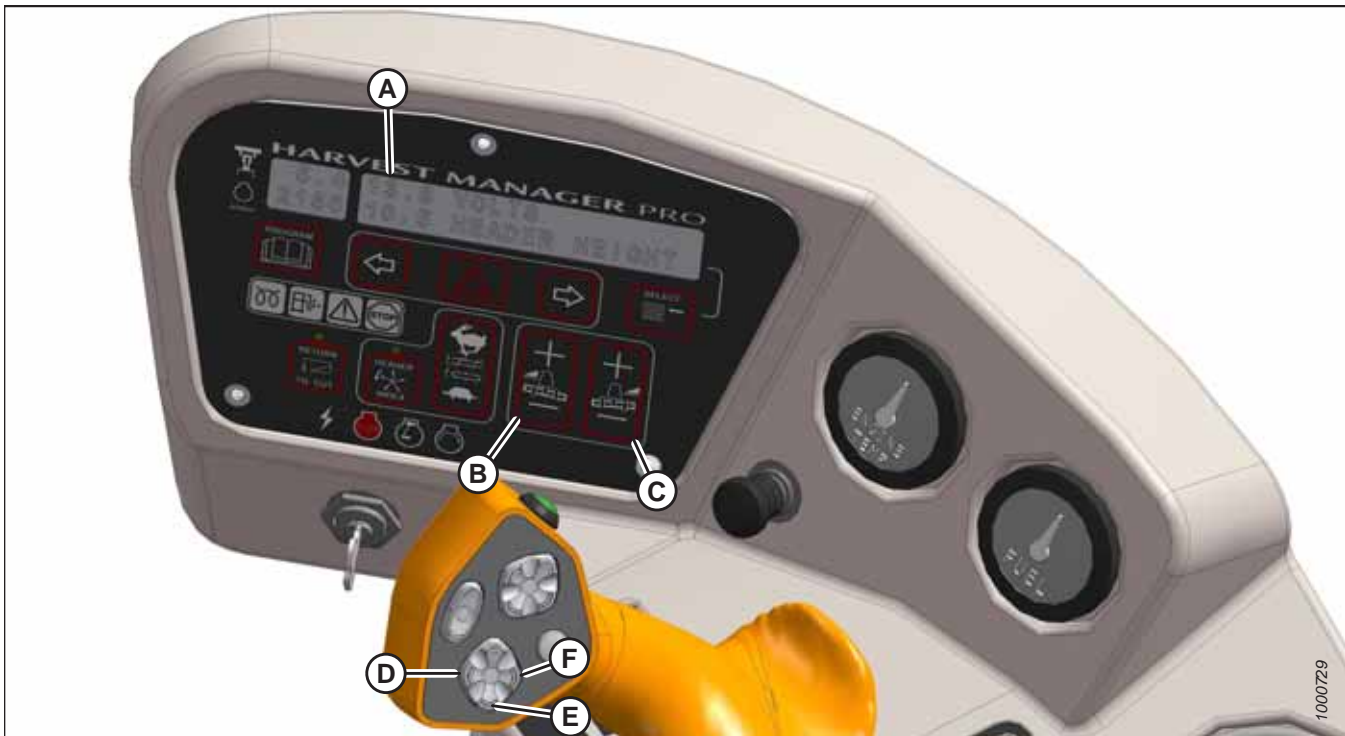
Figure 4.74: Cab Display Module (CDM) Float Adjustment
