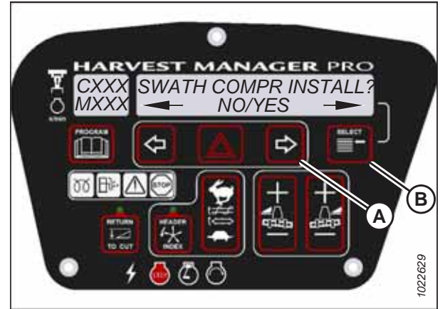
Figure 3.104: Swath Compressor Controls
