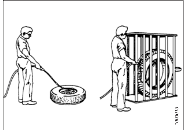
Figure 6.220: Safely Filling a Tire with Air
