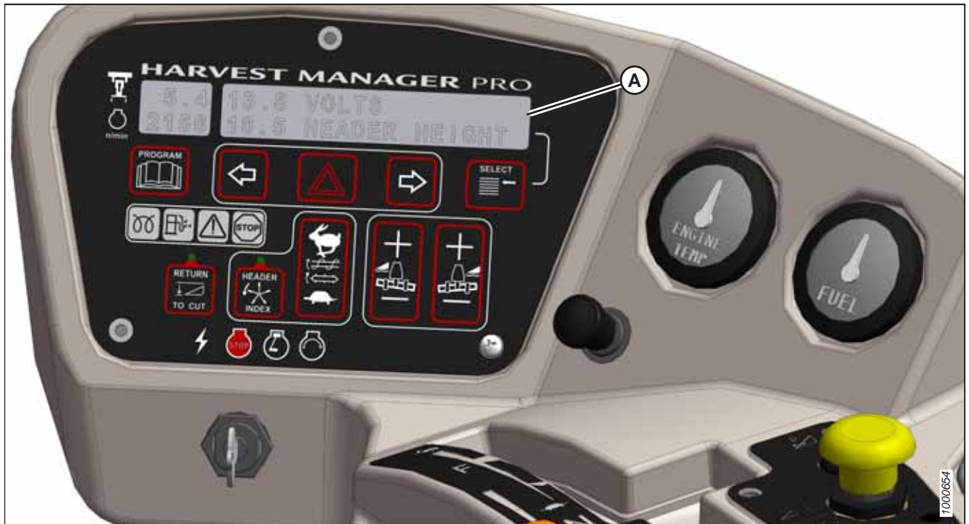
Figure 3.62: CDM Display Warnings and Alarms
