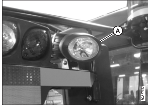
Figure 6.161: New HID Lamp in Place
