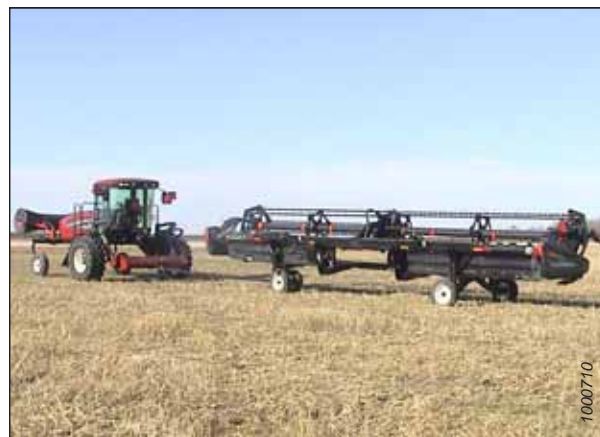
Figure 4.37: Towing a Header
