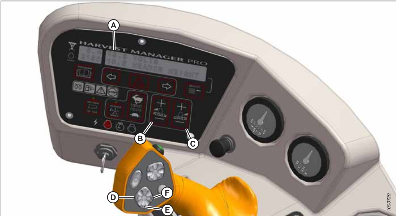
Figure 4.70: Cab Display Module (CDM) Float Adjustment
