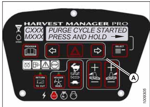
Figure 3.217: Hydraulic Purge Cycle
