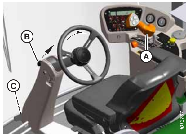
Figure 4.21: Engine-Forward – Seat Faces Engine
