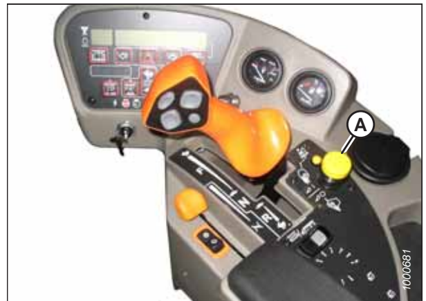
Figure 4.32: Header Drive Switch
