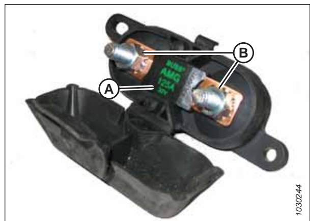
Figure 6.184: 125A Main Fuse
