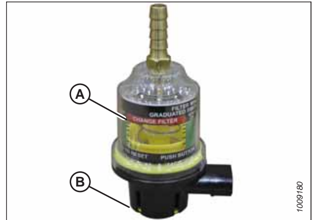
Figure 6.60: Air Filter Restriction Indicator
