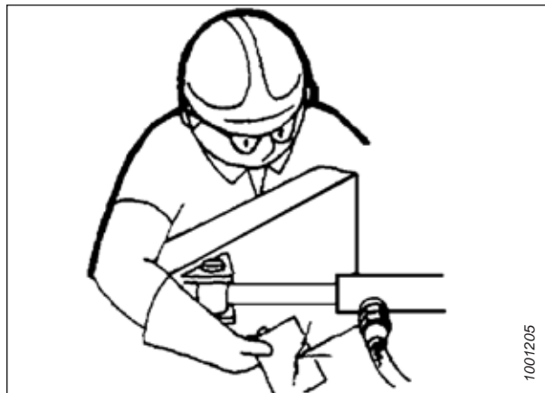
Figure 1.11: Testing for Hydraulic Leaks
