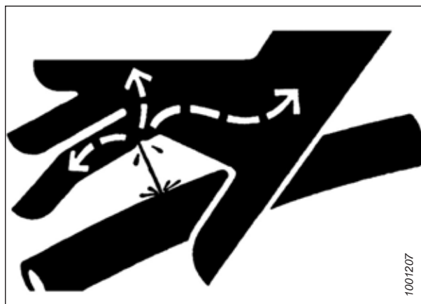
Figure 1.12: Hydraulic Pressure Hazard
