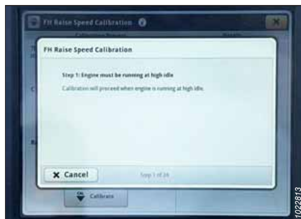
Figure 3.716: John Deere S7 Display – Feeder House Calibration
