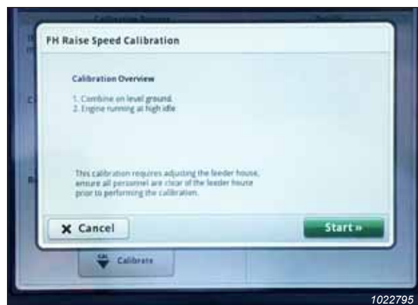
Figure 3.715: John Deere S7 Display – Feeder House Calibration
