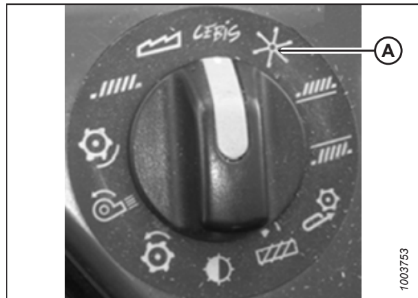
Figure 3.504: CLAAS Combine Rotary Switch
