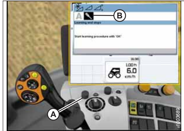
Figure 3.513: CLAAS Combine Display, Console, and Control Handle
