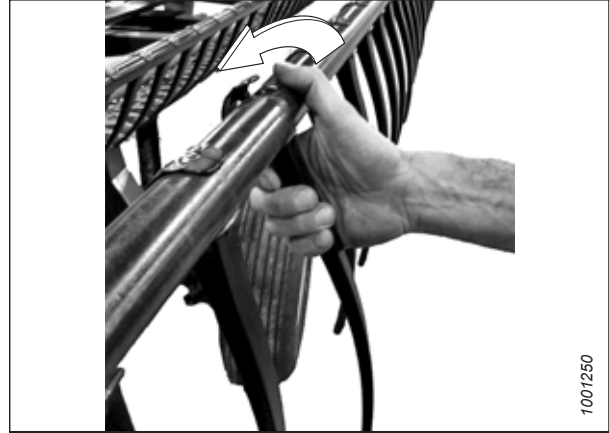
Figure 4.295: Removing Plastic Finger
