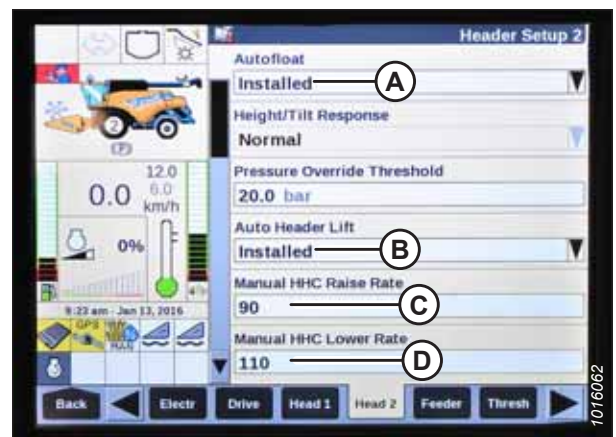
Figure 3.799: New Holland Combine Display
