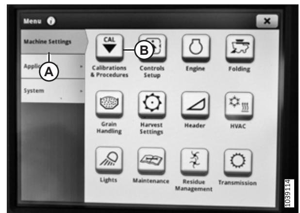
Figure 3.731: John Deere X9 Display – Machine Settings
