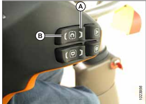
Figure 3.315: John Deere 700 Feeder House Fore-Aft Tilt Controls
