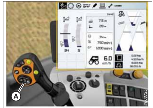
Figure 3.516: CLAAS Combine Display, Console, and Control Handle
