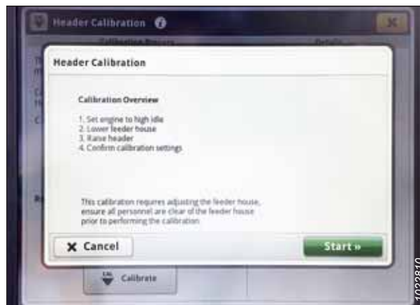
Figure 3.723: John Deere S7 Display – Header Calibration
