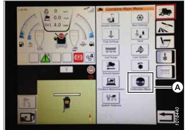
Figure 3.595: Direct Calibration Menu
