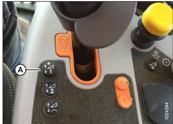
Figure 3.820: New Holland Combine Controls
