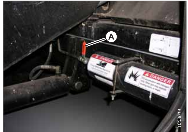
Figure 3.562: Combine Accumulator ON/OFF Switch
