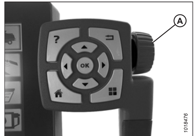
Figure 3.631: Adjustment Wheel on Right of Tyton Terminal
