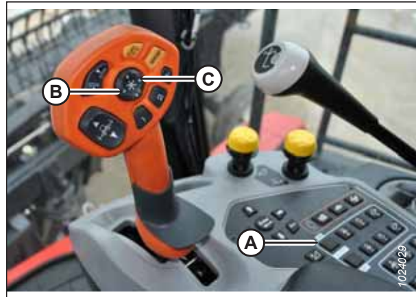
Figure 3.320: Rostselmash Control Handle and Console
