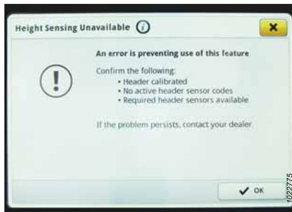
Figure 3.704: John Deere S7 Display – Height Sensing Error Message
