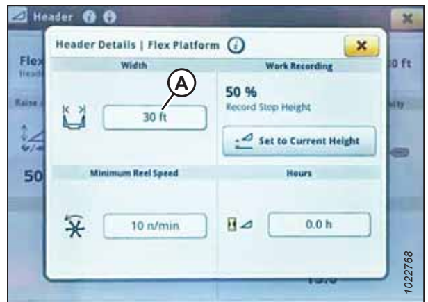
Figure 3.697: John Deere S7 Display – Header Details Window
