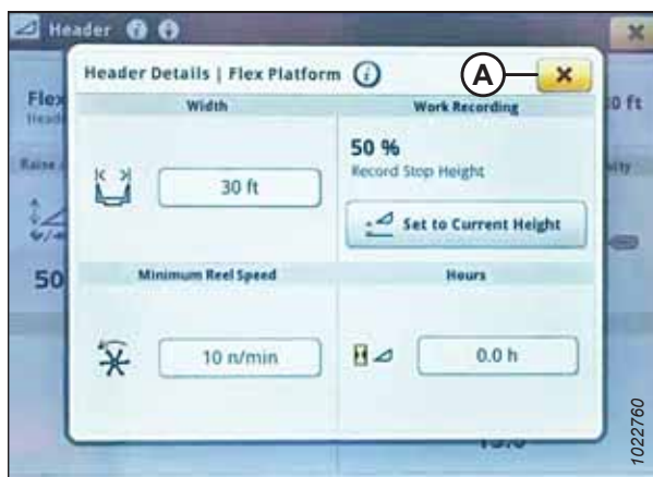
Figure 3.699: John Deere S7 Display – Header Details Dialog Box
