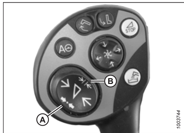
Figure 3.509: CLAAS Control Handle Buttons
