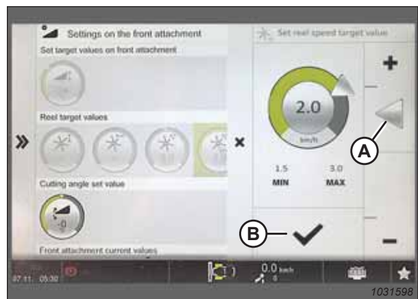
Figure 3.550: Reel Speed Target Value Page
