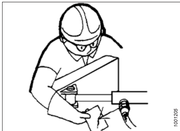
Figure 4.2: Testing for Hydraulic Leaks
