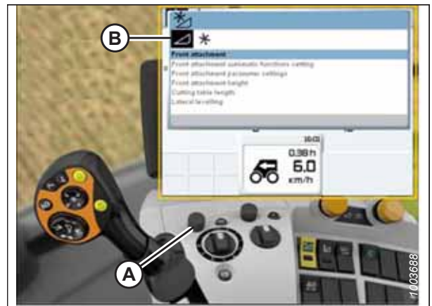
Figure 3.511: CLAAS Combine Display, Console, and Control Handle
