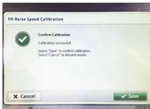
Figure 3.717: John Deere S7 Display – Feeder House Calibration
