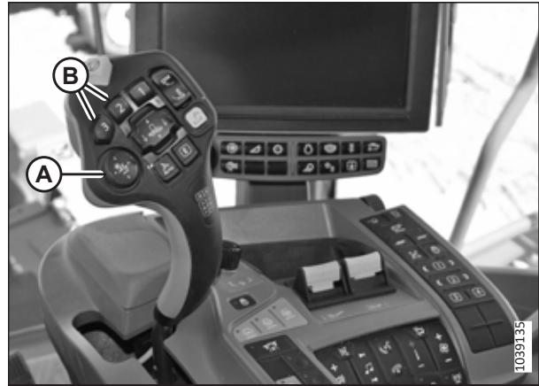
Figure 3.753: John Deere X9 – Multi-Function Lever
