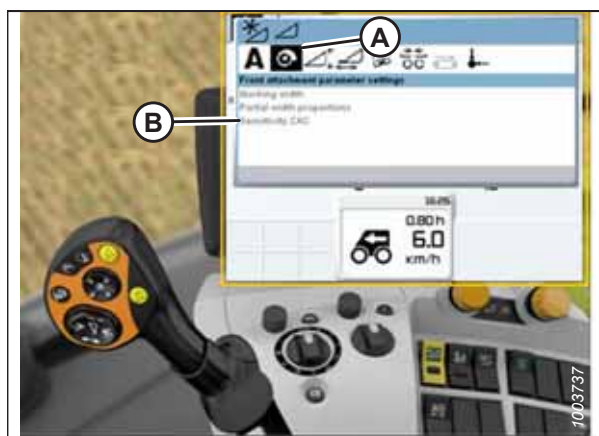
Figure 3.518: CLAAS Combine Display, Console, and Control Handle
