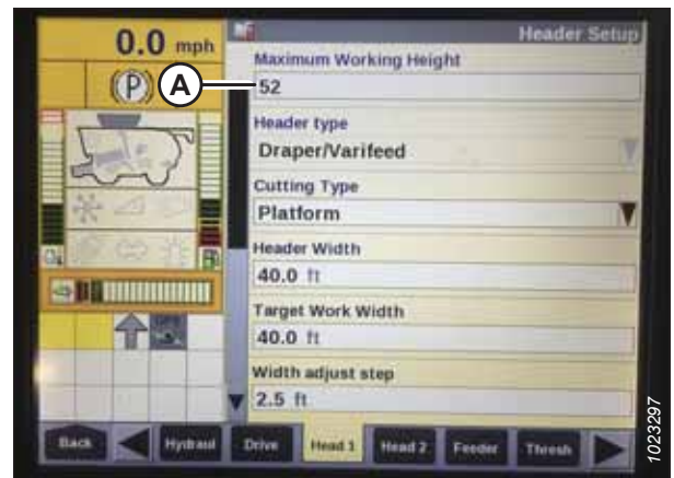
Figure 3.438: Case Combine Display – Header Setup Page
