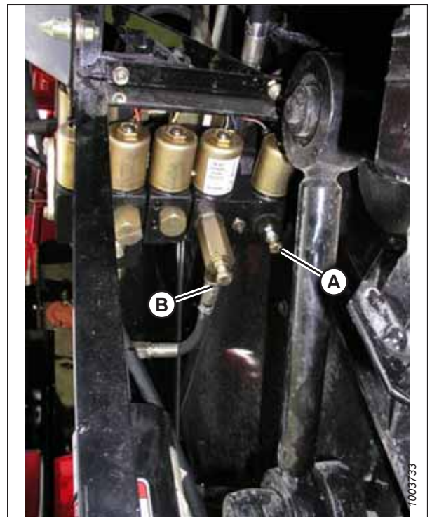
Figure 3.563: Header Raise and Lower Adjustable Restrictors
