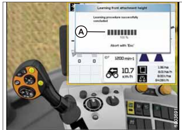
Figure 3.515: CLAAS Combine Display, Console, and Control Handle
