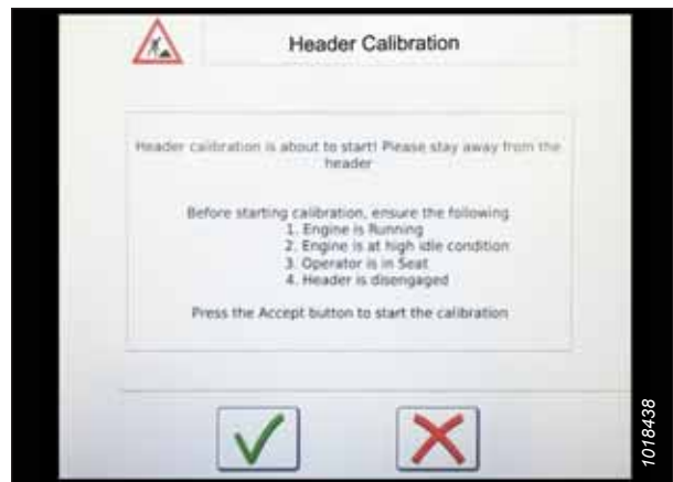
Figure 3.622: Header Calibration Warning
