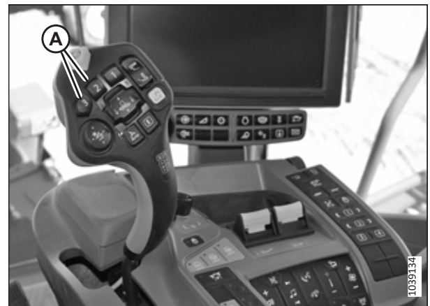
Figure 3.752: John Deere X9 – Multi-Function Lever
