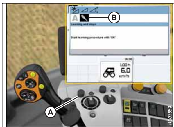
Figure 3.527: CLAAS Combine Display, Console, and Control Handle
