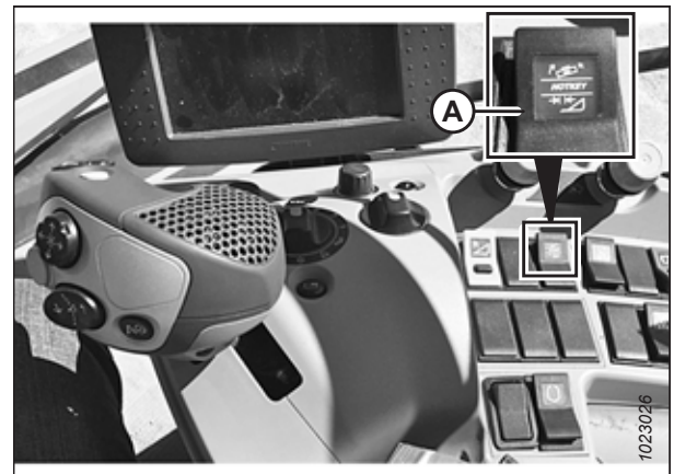
Figure 3.239: Multi-Function Trigger Rocker Switch
