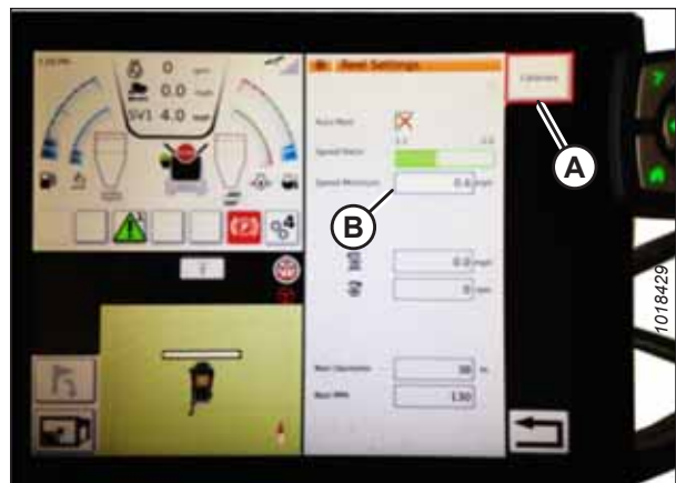
Figure 3.580: Reel Settings Calibration
