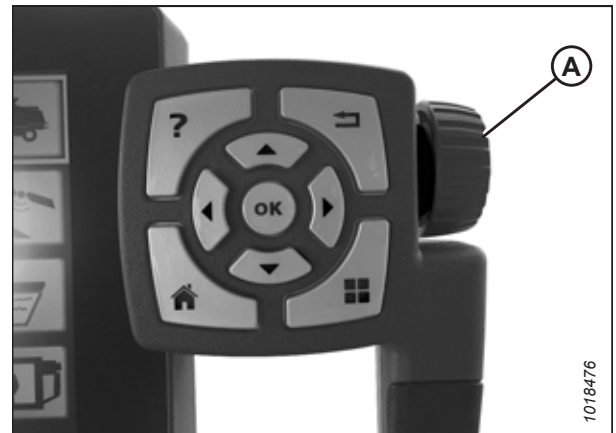
Figure 3.601: Adjustment Wheel on Right Side of Tyton Terminal
