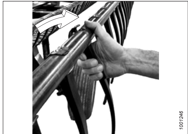
Figure 4.296: Installing Plastic Finger
