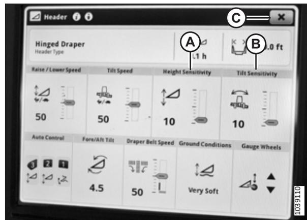
Figura 3.729: Display CommandCenter™ – Schermata HEADER (Testata)
