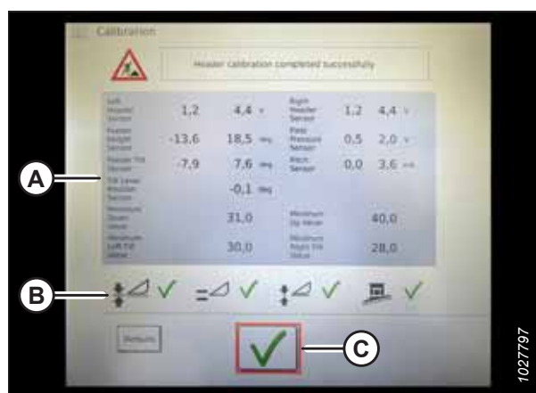
Figure 9.229: Completed Calibration Page
