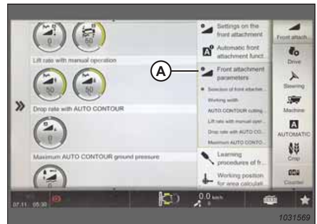
Figure 9.149: Front Attachment Parameters Page
