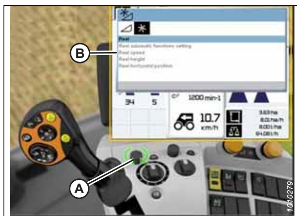
Figure 9.121: CLAAS Combine Display, Console, and Control Handle
