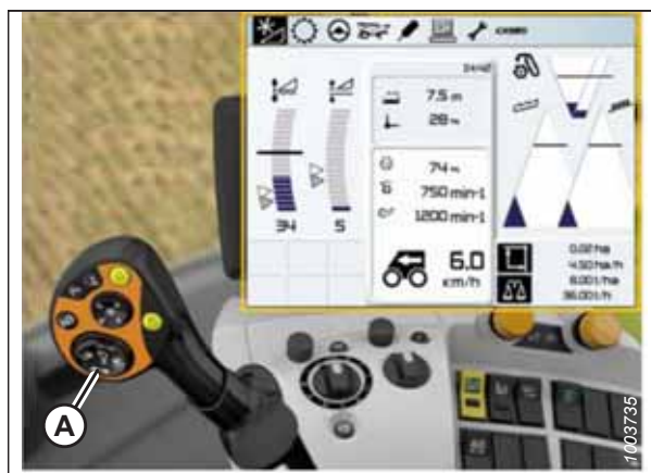
Figure 9.116: CLAAS Combine Display, Console, and Control Handle
