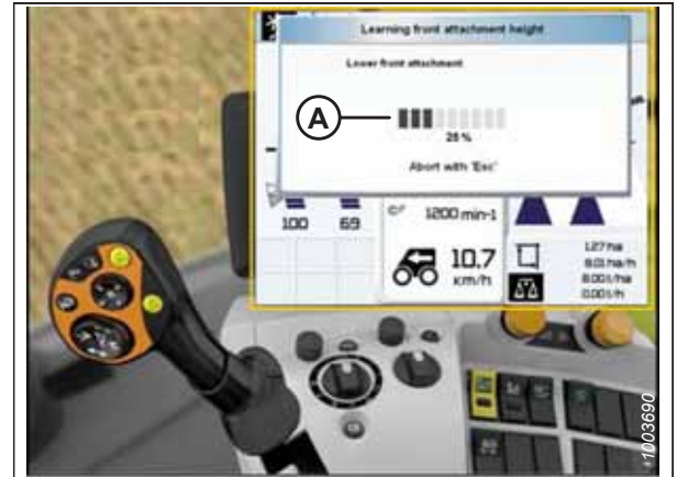
Figure 9.113: CLAAS Combine Display, Console, and Control Handle
