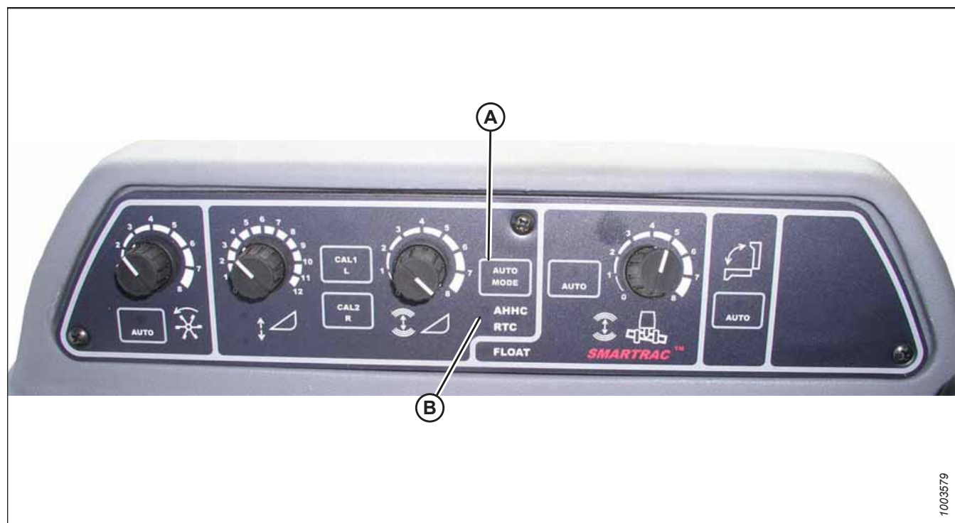
Figure 9.162: Combine Auto Header Height Controls
