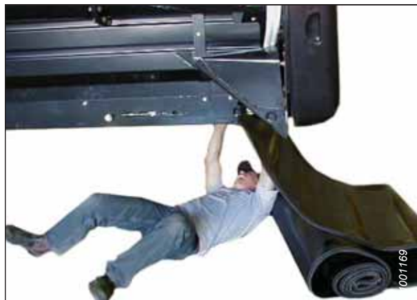
Figure 5.227: Installation du tapis
