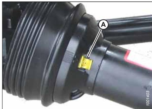
Figure 4.60: Protection de transmission
