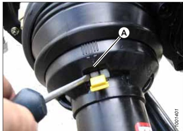
Figure 4.59: Protection de transmission
