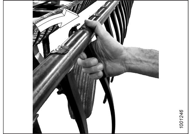
Figure 5.285: Installing Plastic Finger
