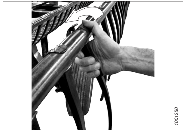
Figure 5.284: Removing Plastic Finger
