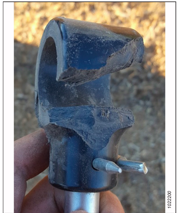
Figure 5.76: Broken Finger Holder
