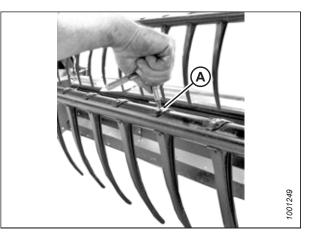
Figure 4.291: Installing Plastic Finger
