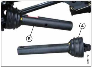
Figure 4.54: Separated Driveline
