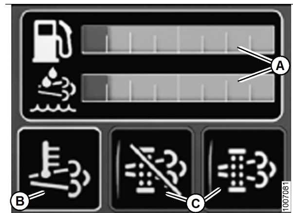
Figure 4: Diesel Exhaust Fluid (DEF) Display Monitor
