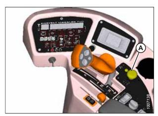
Figure 4.32: Header Drive Switch
