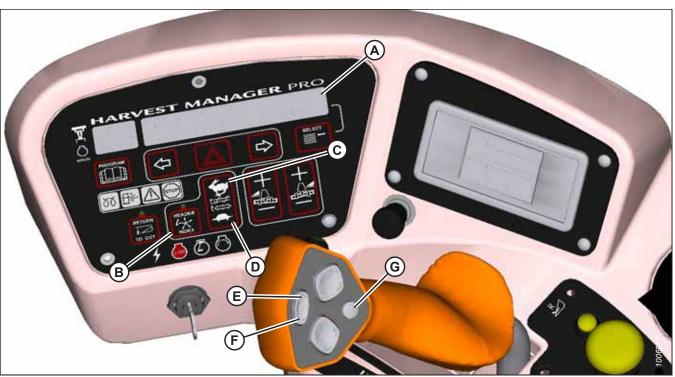
Figure 4.281: Operator Console
