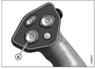
Figure 4.168: Ground Speed Lever
