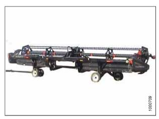
Figure 4.39: Header in Transport Mode
