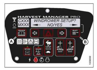
Figure 3.122: M155 CDM Programming Buttons Shown – M155*E4* Similar
