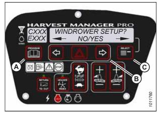
Figure 3.123: M155E4 Cab Display Module
