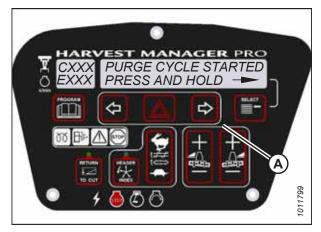
Figure 3.233: Hydraulic Purge Cycle
