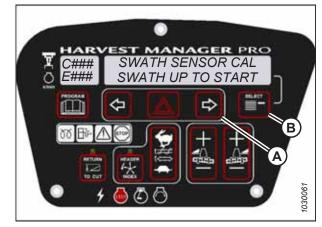
Figure 3.175: Swath Compressor Sensor Calibration
