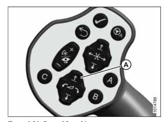
Figure 4.64: Ground Speed Lever
