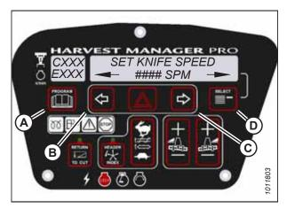
Figure 3.96: Knife Speed Setting
