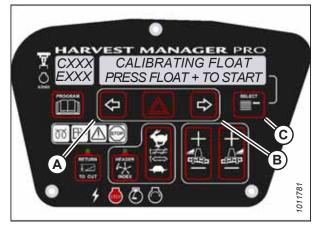
Figure 3.171: Header Float Display
