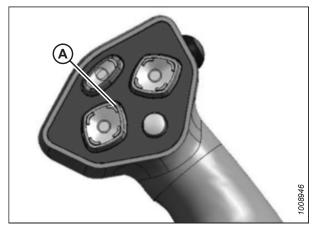
Figure 4.122: Ground Speed Lever
