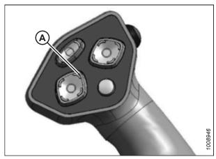
Figure 4.210: Ground Speed Lever (GSL)
