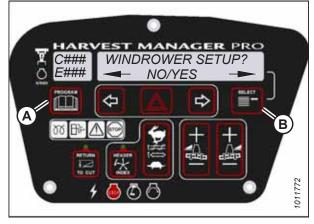
Figure 3.80: Windrower Setup Display
