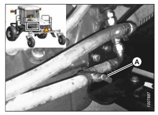
Figure 3.33: Heater Shut-Off Valve
