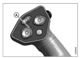
Figure 4.162: Ground Speed Lever
