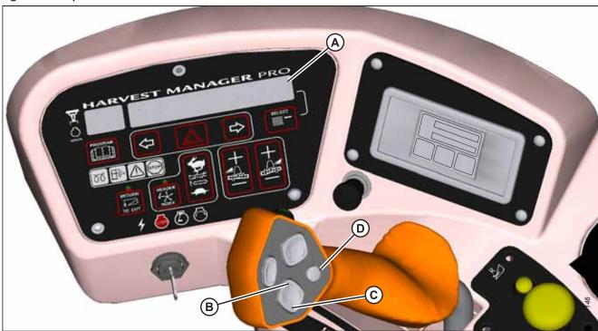
The cab display module (CDM) displays the current header height setting on the lower line of DISPLAY (A). The reading will range between 00.0 and 10.0, with 00.0 representing the header sitting flush with the ground, and 10.0 indicating that the header is at its maximum height. Use HEADER UP button (B) and HEADER UP button (C) to change the height of the header.
