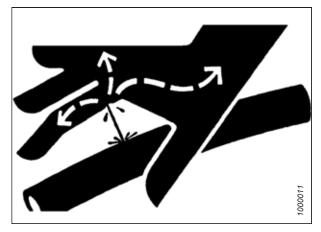
Figure 5.196: Hydraulic Pressure Hazard
