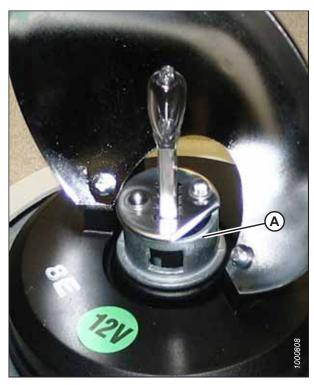
Figure 5.177: Beacon Lamp Assembly
