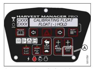
Figure 3.173: Negative Header Float Display
