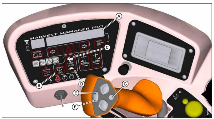
Figure 4.282: Operator's Console
