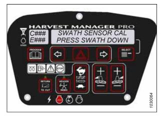
Figure 3.177: Swath Compressor Sensor Calibration
