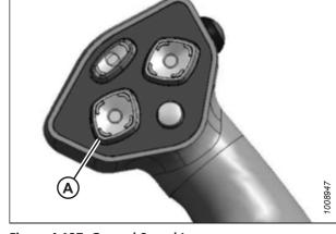
Figure 4.127: Ground Speed Lever
