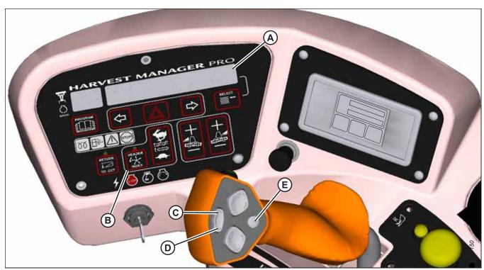
Figure 4.284: Operator Console
