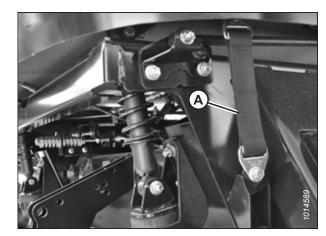
Figure 5.27: Cab Suspension
