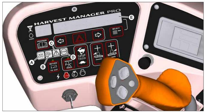
Figure 3.77: CDM Engine Warning Lights
