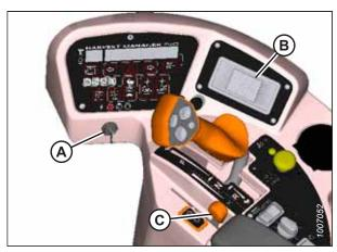
Figure 3.50: Engine Controls and DEF Display Module
