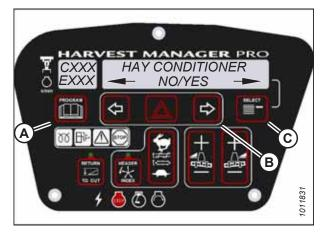
Figure 3.124: M155E4 Cab Display Module
