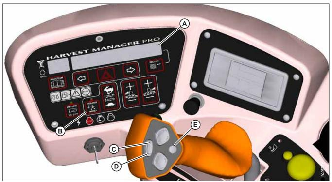
Figure 4.287: Operator Console
