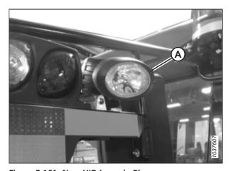
Figure 5.161: New HID Lamp in Place
