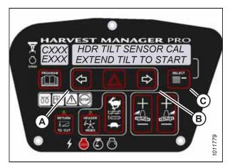
Figure 3.166: Header Tilt Calibration
