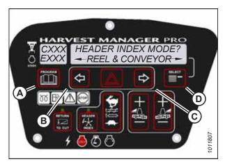
Figure 3.104: Header Index Mode
