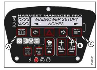
Figure 3.119: M155 Programming Buttons Shown – M155*E4* Similar
