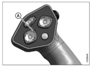
Figure 4.147: Ground Speed Lever
