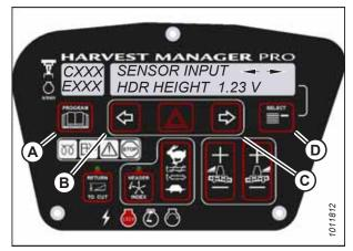
Figure 3.188: Header Sensors
