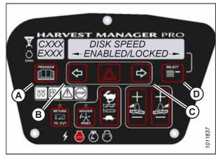
Figure 3.153: Disc Speed Control Lock
