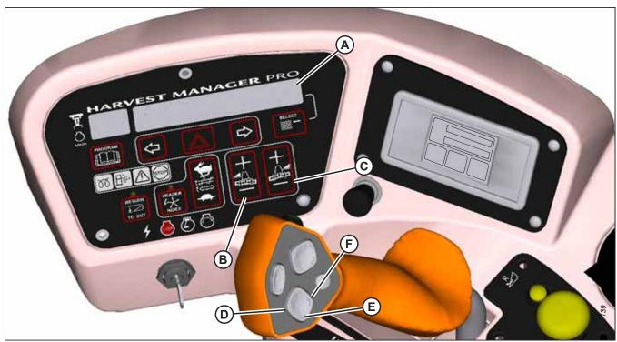
Figure 4.67: Cab Display Module (CDM)
