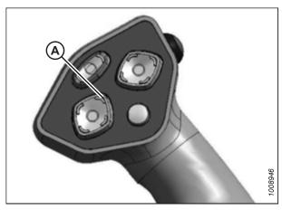
Figure 4.130: Ground Speed Lever (GSL)
