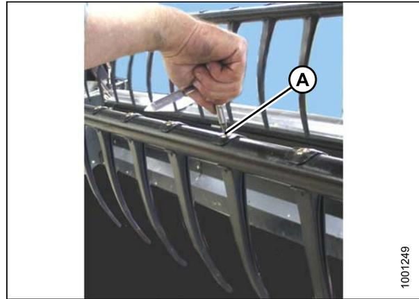
Figure 6.261: Installation des doigts
