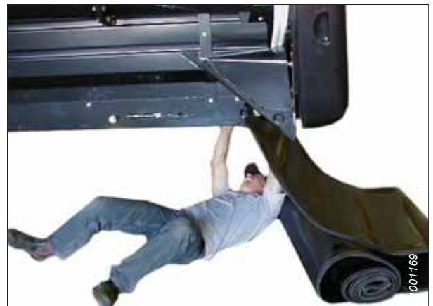
Figure 6.220: Installation du tapis
