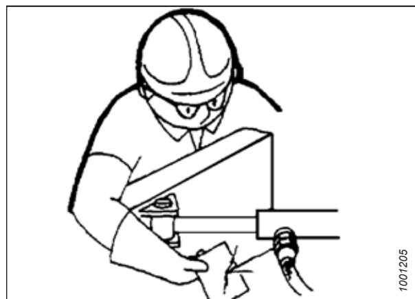
Figure 6.3: Test de fuites hydrauliques
