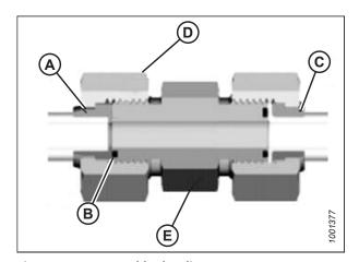
Figure 8.15: Raccord hydraulique
