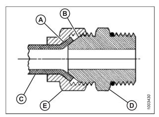
Figure 8.10: Raccord hydraulique
