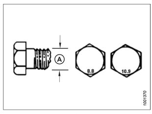
Figure 8.6: Grades des boulons
