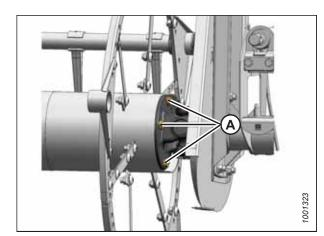
Figure 5.251: Joint universel
