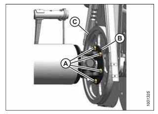
Figure 5.240: Joint universel
