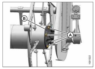
Figure 5.249: Joint universel
