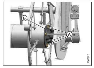
Figure 5.239: Joint universel
