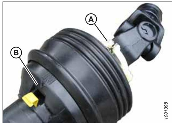
Figure 5.21: Protection de transmission
