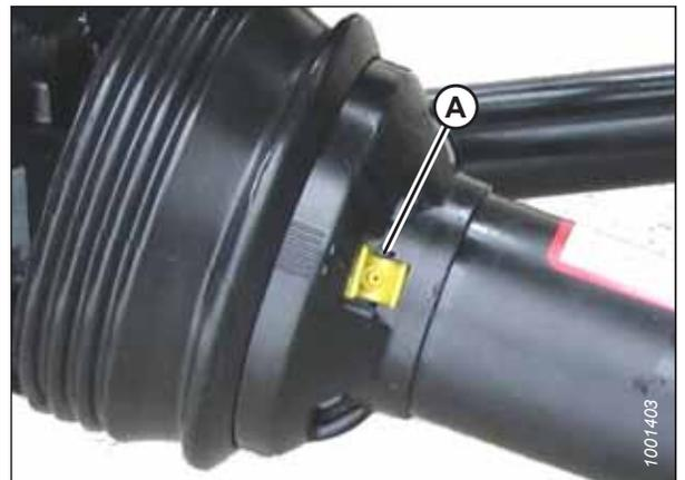
Figure 5.24: Protection de transmission
