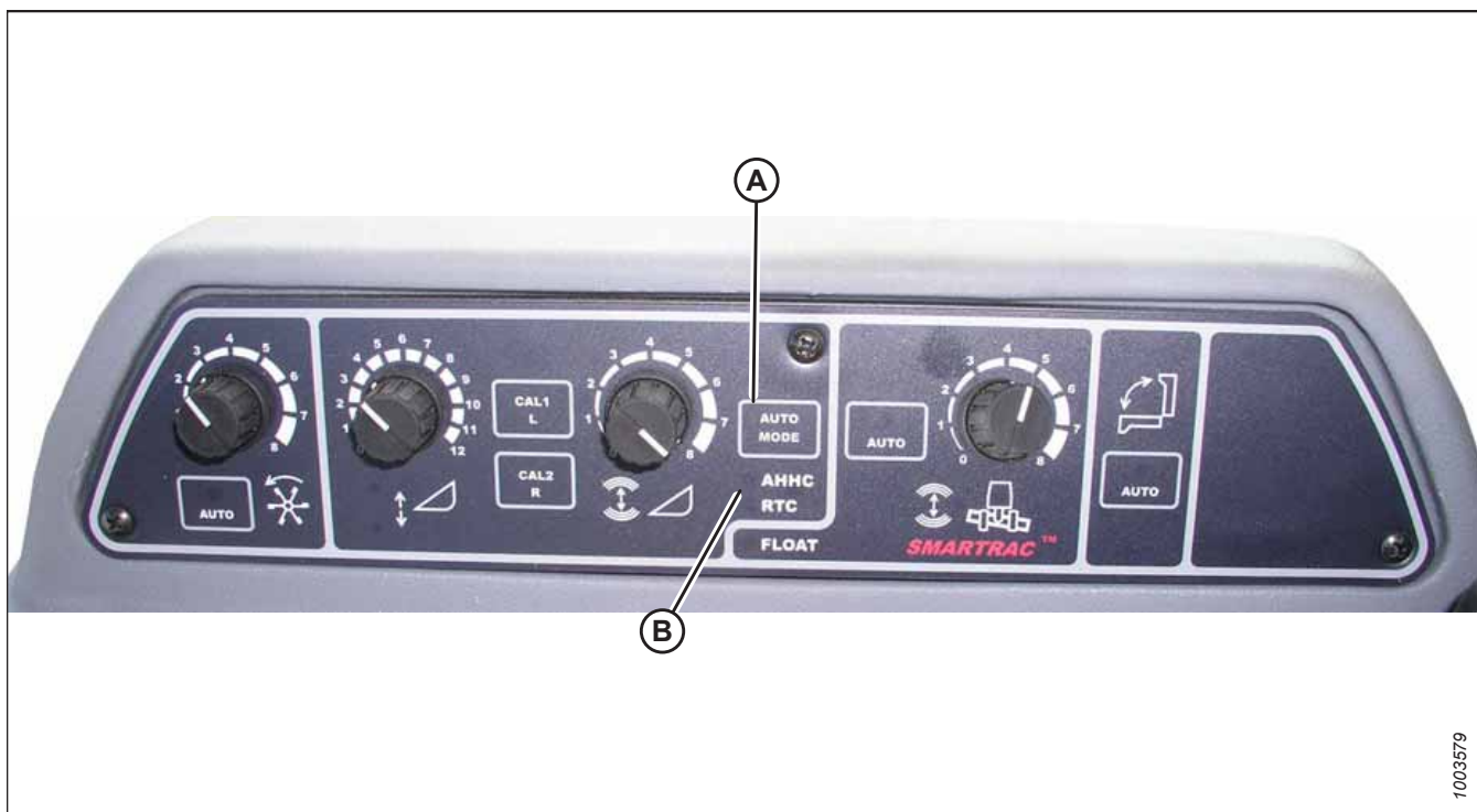
Figure 4.132: Combine Auto Header Height Controls
