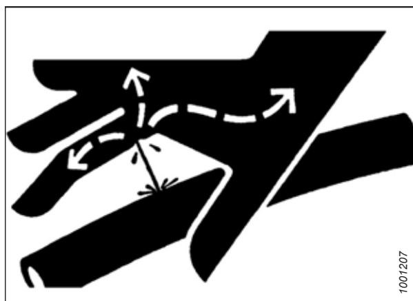
Figure 6.2: Hydraulic Pressure Hazard
