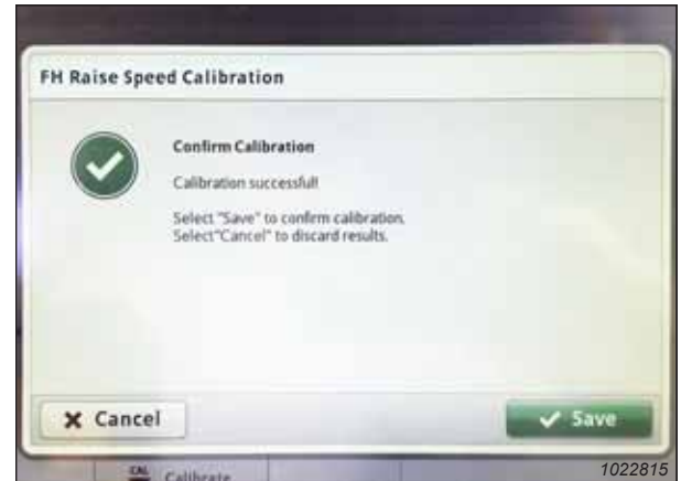
Figure 4.269: John Deere S7 Display – Feeder House Calibration
