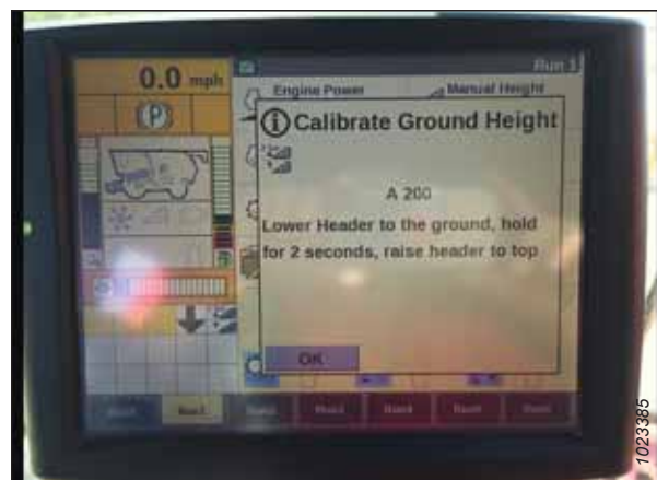
Figure 4.32: Calibrating Auto Header Height
