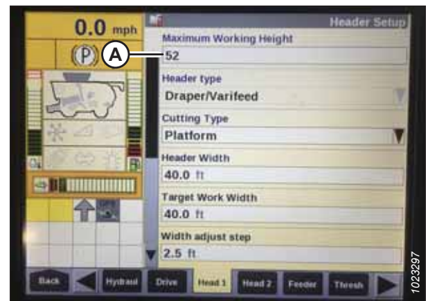
Figure 4.37: Case Combine Display – Header Setup Page
