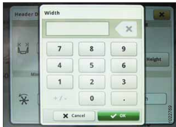
Figure 4.251: John Deere S7 Display – Setting Header Width
