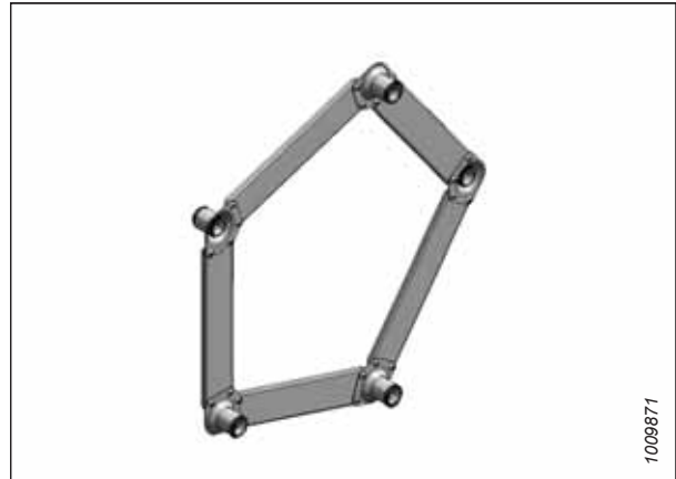
Figure 7.6: Five-Bat Reinforcing Kit Shown – Six-Bat Reinforcing Kit Similar
