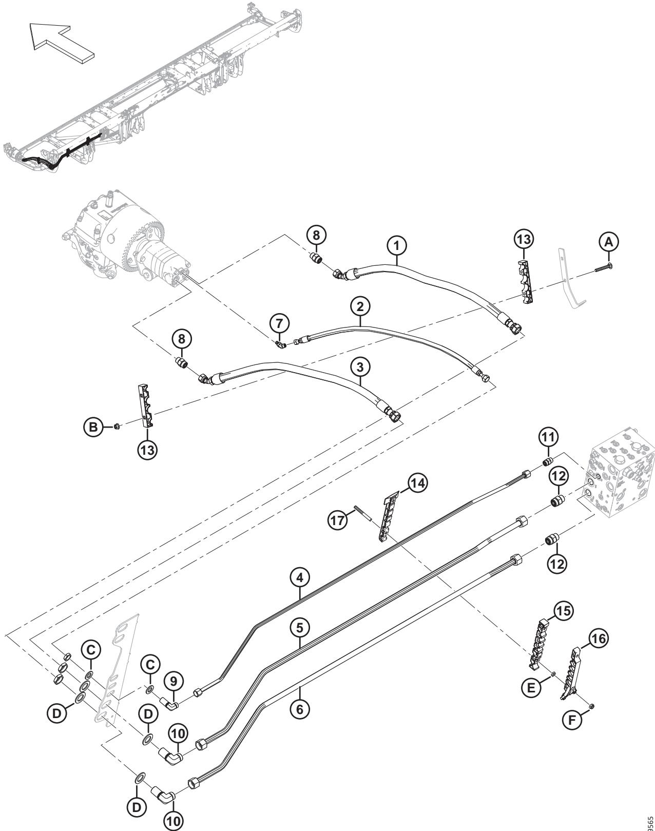
**SYSTÈME HYDRAULIQUE – ENTRAÎNEMENT COUTEAU, COUTEAU SIMPLE ET COUTEAU DOUBLE, CÔTÉ GAUCHE (FD225, FD230, FD235, FD240, FD241 ET FD245)**
