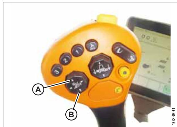
Figura 3.462: Alavanca de controle John Deere
