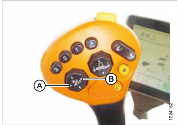
Figura 3.90: Alavanca de controle John Deere
