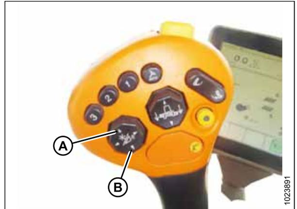
Figura 3.382: Alavanca de controle John Deere
