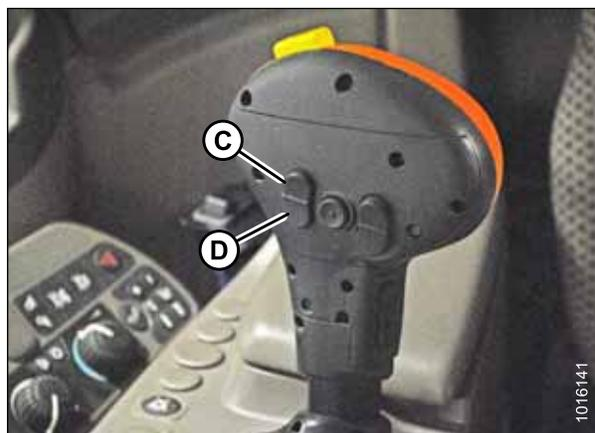
Figura 3.366: Alavanca de controle John Deere
