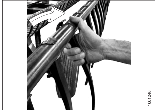
Figure 5.234: Installing Plastic Finger
