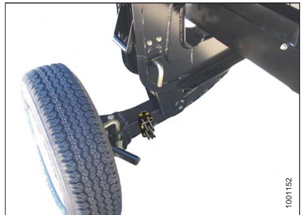
Figure 3.534: Left Wheel in Transport Position
