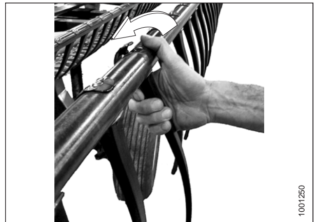
Figure 5.233: Removing Plastic Finger
