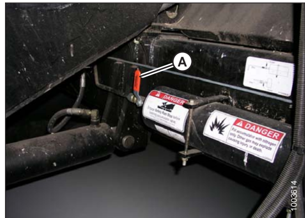
Figure 3.272: Combine Accumulator ON/OFF Switch
