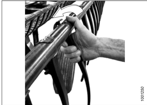
Figure 5.168: Removing Plastic Fingers
