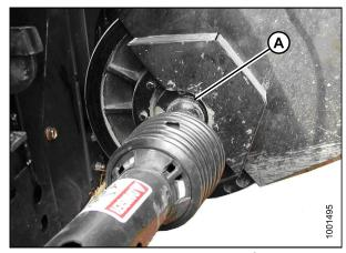
Figure 5.110: Disconnect driveshaft
