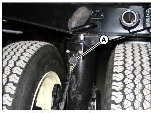
Figure 4.86: Wiring connector
