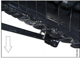
Figure 7.105: Downward adjustment
