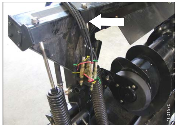
Figure 3.142: Store and secure hoses
