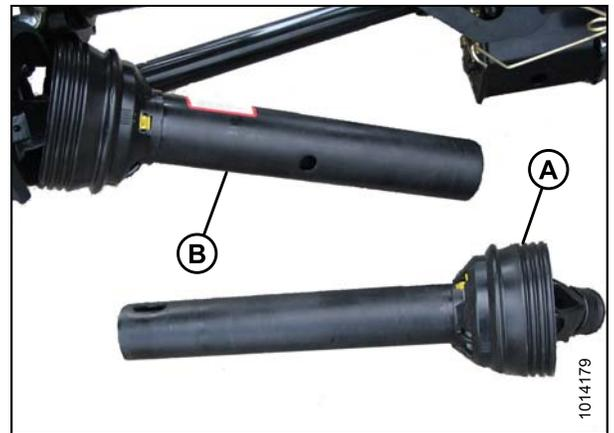
Figure 5.43: Separated Driveline
