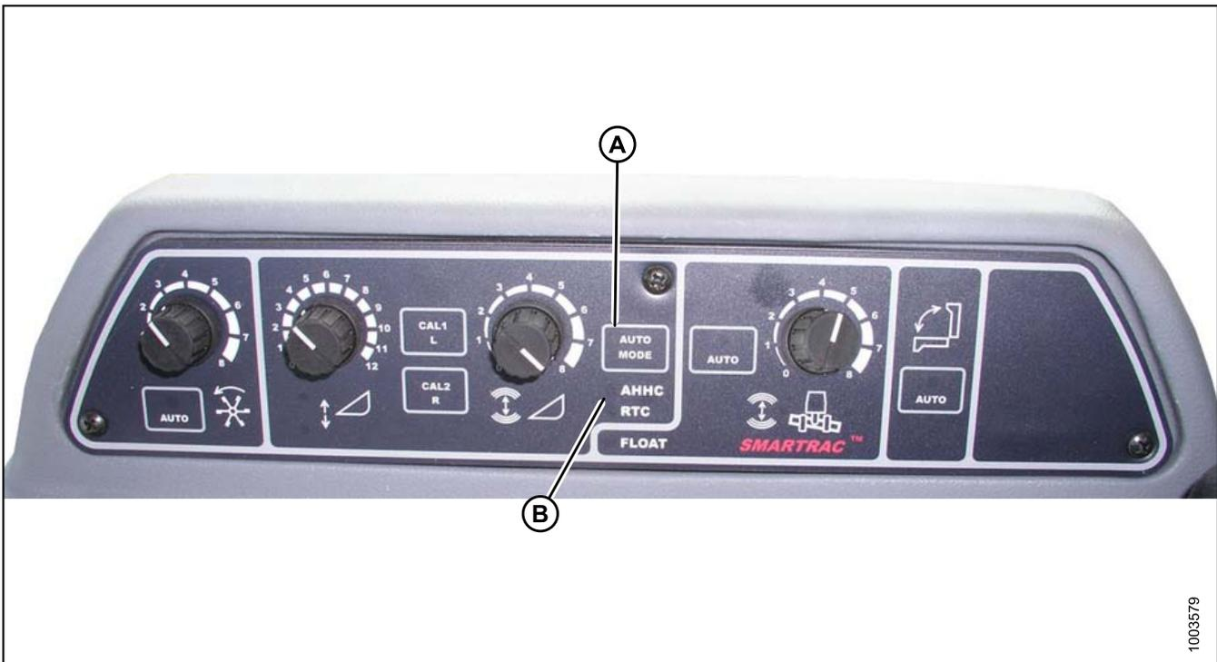
**Figure 3.159: Combine Auto Header Height Controls**
