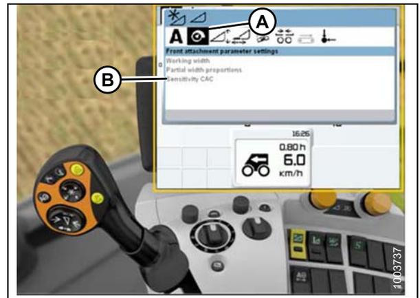
Figure 3.319: Lexion Combine Display, Console, and Joystick Lever
