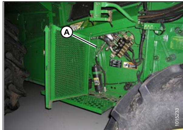
Figure 3.216: Accumulator Shut-off
