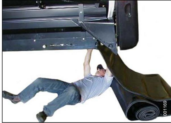
Figure 5.213: Installing Draper
