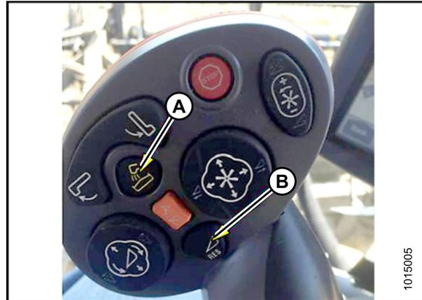
**Figure 3.344: New Holland Combine Controls**
