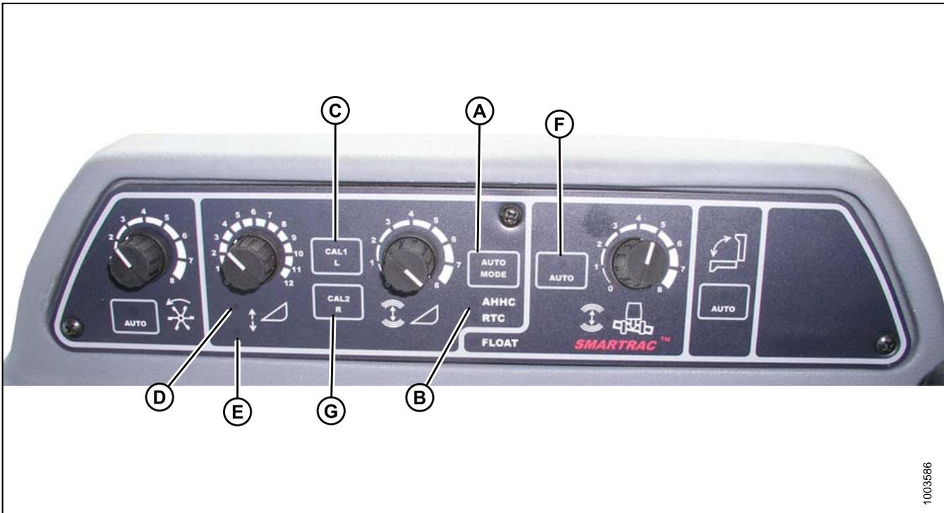
**Figure 3.161: Combine Auto Header Height Controls**
