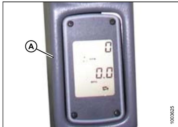
**Figure 3.167: Tachometer**
