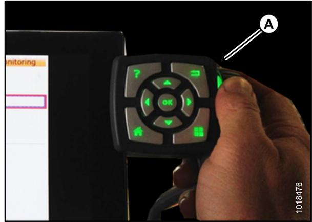
Figure 3.201: Scroll Wheel for Adjustments
