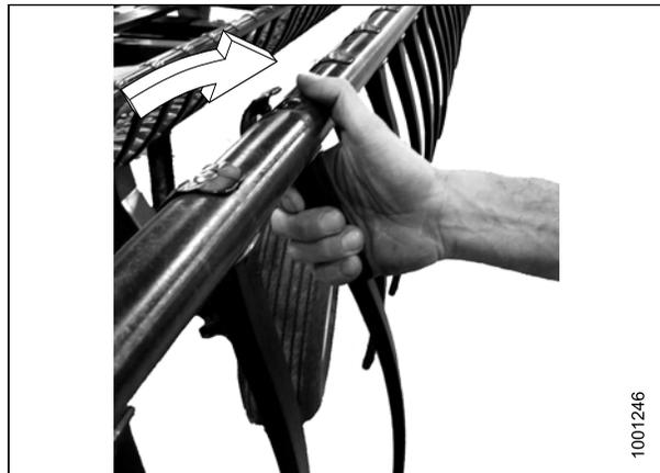
Figure 5.266: Installing Finger
