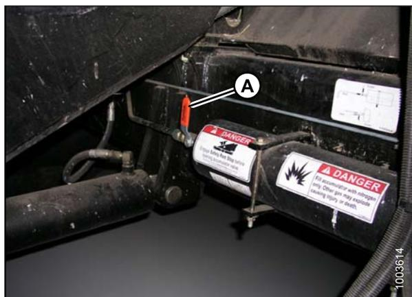
**Figure 3.162: Combine Accumulator ON/OFF Switch**
