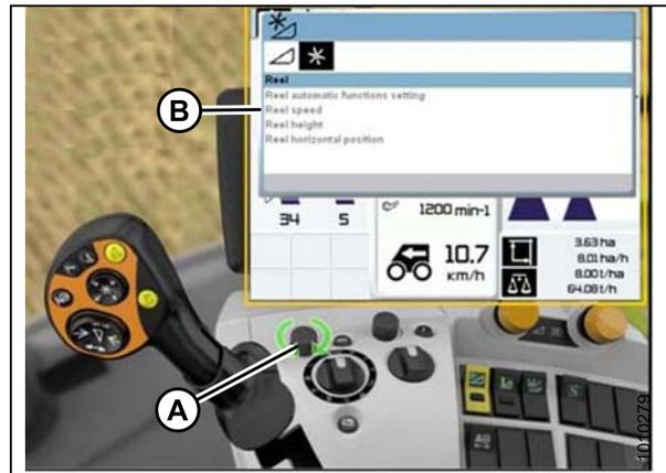
Figure 3.322: Lexion Combine Display, Console, and Joystick
