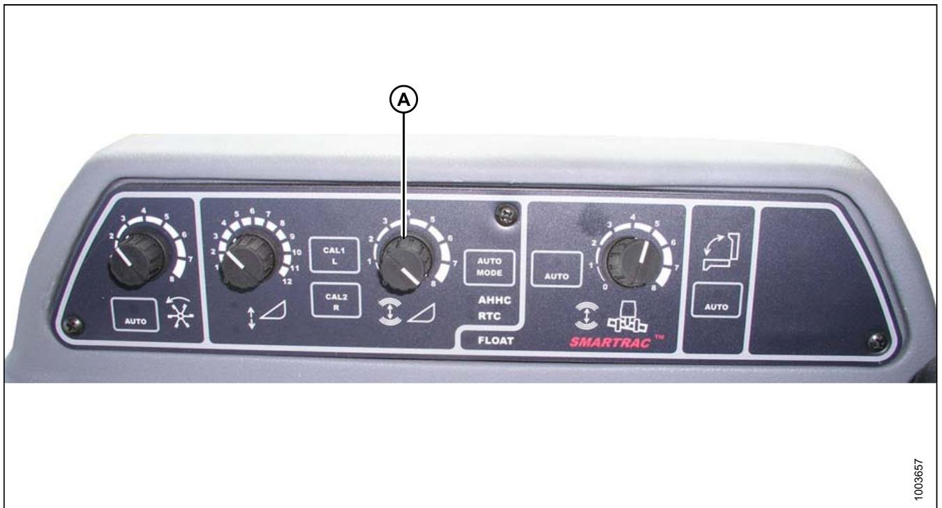
Figure 3.166: Auto Header Height Control Console
