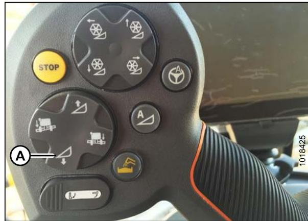
Figure 3.190: Header Down Switch
