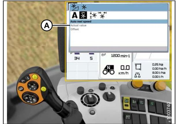
Figure 3.323: Lexion Combine Display, Console, and Joystick
