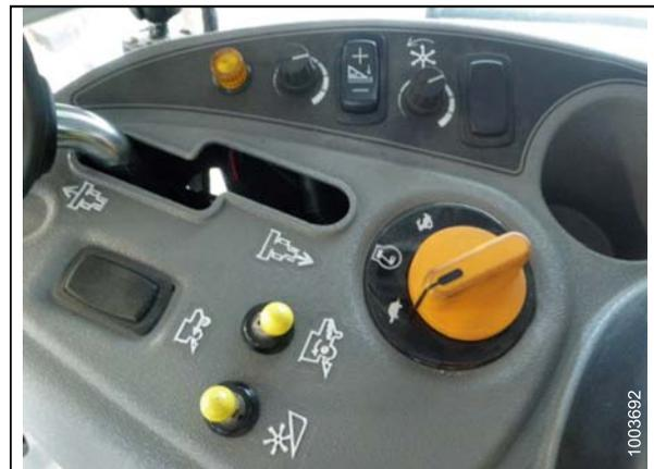
**Figure 3.143: Height Adjustment Knob on the Combine Control Console**
