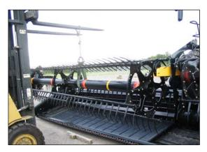
1. Support inboard end of right reel with a front end loader and nylon slings (or equivalent set-up).
