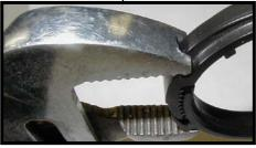
3. Tighten clamp with modified channel lock pliers (K) so that finger pressure will <u>not</u> move clamp.
