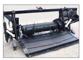
There is a drain plug at the bottom of each side frame.
