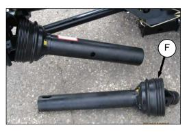
Lift combine end of driveline (F) from hook, and extend driveline until it separates. Hold adapter end of driveline to prevent it from dropping and hitting the ground.
