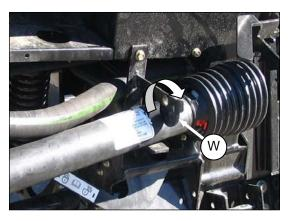
Rotate disc (W) on adapter driveline storage hook, and remove driveline from hook.
