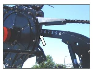
Adjust fore-aft reel position so that back end of cam disc is approximately between 4 and 5 on the arm decal.
