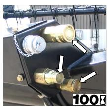
LUBRICATE WITH WD40® OR EQUIVALENT
