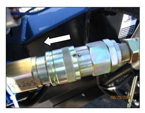
Push hose connector onto mating receptacle until collar on receptacle snaps into lock position.
