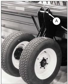
c. Remove pin (A), and pull wheel assembly towards rear of header. Store pin (A) in hole at top of leg.
