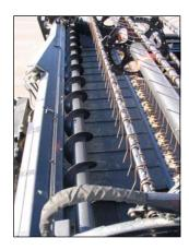
The cross auger helps deliver very bulky crops across the header onto the windrow or into the combine.
