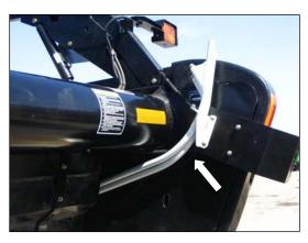
b. Store both rods on the inboard side of the right endsheet.
