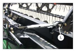
I. Remove pin (L) to release link. Replace pin.
