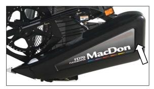
d. Push in shield where shown (opposite latch), and shield will self-latch.
