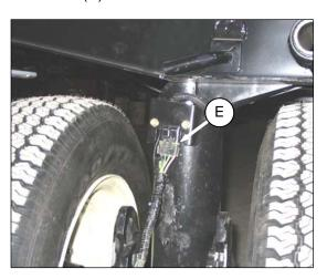
3. Disconnect wiring connector (E) at front wheel.
