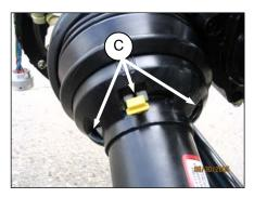
b. Push guard onto ring until locking ring is visible in slots (C).
