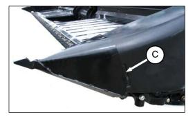
c. To close shield, lift latch (B), and swing shield forward until front engages crop divider (C).
