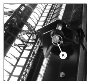
2. Remove pin (K), and the prop under link.
