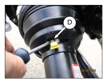
c. Rotate ring (D) clockwise with a screwdriver to lock ring in guard.
