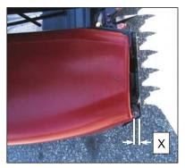
d. Adjust the endshield to achieve the gap 'X' between the front end of shield and header frame in accordance with the following chart.
