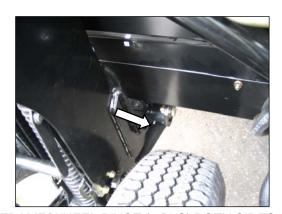
FRAME/WHEEL PIVOT (1 PLC) BOTH SIDES
