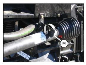
I. Rotate disc (M) on adapter driveline storage hook, and remove driveline from hook.
