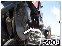
REEL SHAFT RH BEARING (1 PLC)
