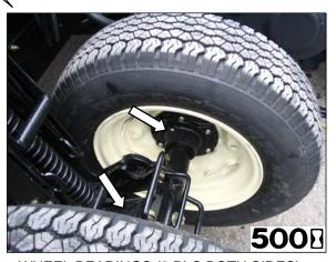
WHEEL BEARINGS (2 PLC BOTH SIDES)
