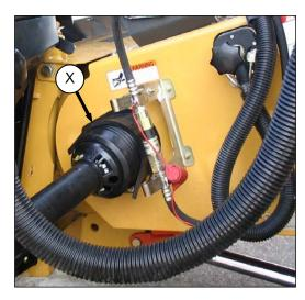
j. Attach driveline to combine output shaft (X).
