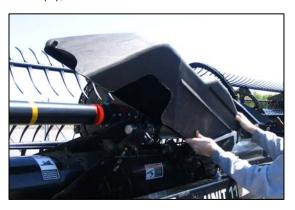
b. Rotate upward until inboard end can be lifted off.
