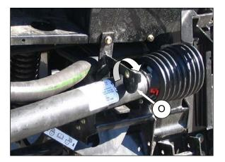
j. Rotate disc (O) on adapter driveline storage hook, and remove driveline from hook.
