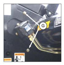
f. Tighten the two bolts (G) on the endsheet.
