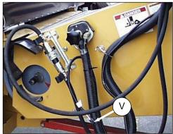
h. If adapter is equipped with reel fore-aft/header tilt selector, connect harness (U) to combine harness (V). (shown in previous column).
