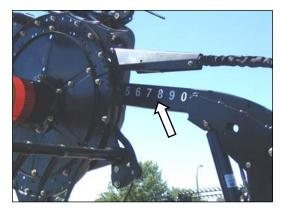
A gauge decal is provided on the reel right support arm for identifying a preferred position. The back edge of the reel cam disc is the gauge indicator.
