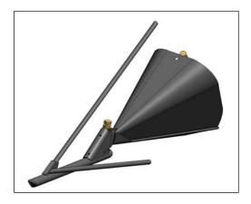
Optional special rice dividers can be installed and used when required. See Section 12.15 RICE DIVIDER KIT.
