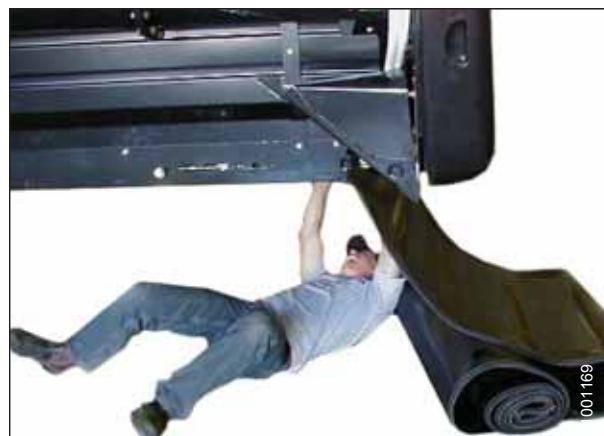
Figure 5.107: Installation du tapis
