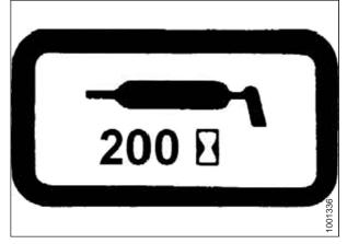
Figure 5.11: Greasing Interval Decal
