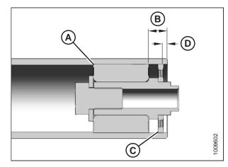
Figure 5.132: Drive Roller Bearing
