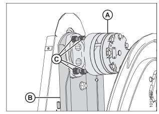
Figure 5.226: Reel Drive Motor
