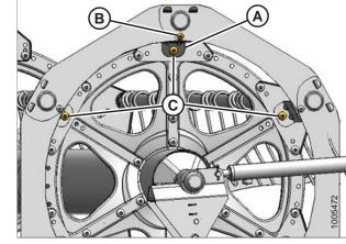
Figure 5.201: Reel Endshield Supports
