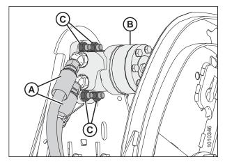
Figure 5.224: Reel Motor and Hoses
