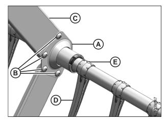
Figure 5.174: Tine Tube Support
