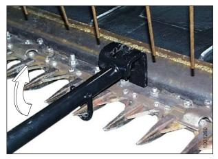
Figure 5.33: Upward Adjustment
