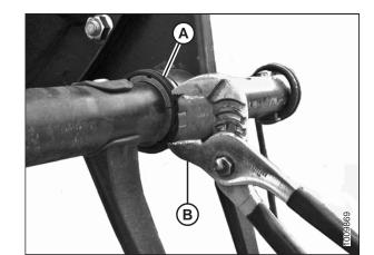
Figure 5.182: Clamp on Bushing
