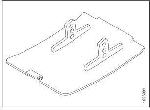
Figure 6.17: Steel Skid Shoe
