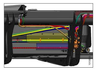
Figure 6.25: Hydraulic Deck Shift
