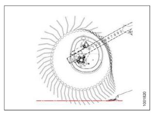
Figure 3.51: Finger Profile – Cam Position 2
