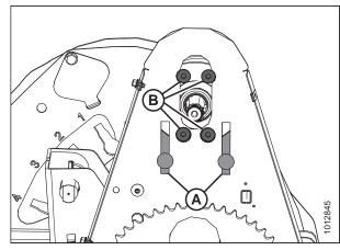
**Figure 5.225: Reel Drive Motor Mounting Holes**
