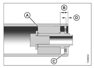
Figure 5.125: Idler Roller Bearing
