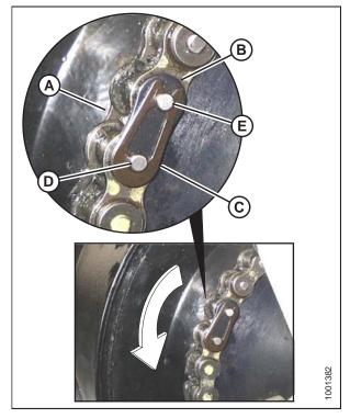
Figure 5.1: Chain Link Connector
