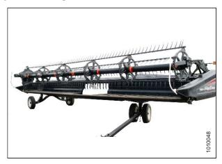
Figure 6.14: Stabilizer Wheels and Slow Speed Transport
