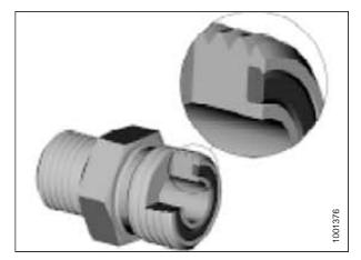
Figure 8.9: Hydraulic Fitting
