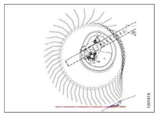
Figure 3.50: Finger Profile - Cam Position 1
