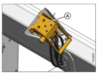
Figure 4.9: Closed Receptacle Cover
