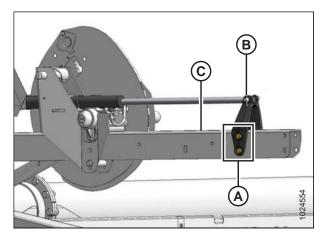
Figure 3.41: Right Reel Arm Cylinder in Aft Position
