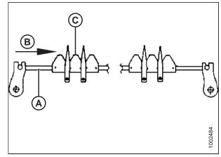
Figure 5.88: Adjusting Timing – Left Side
