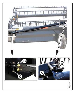
Figure 3.109: Tow-Bar Removal – Left Side
