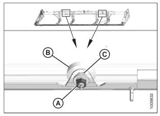
Figure 5.96: Cross-Shaft Support
