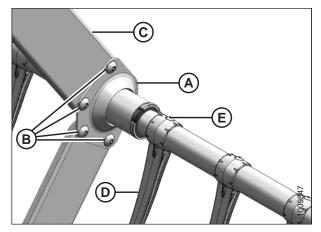
Figure 5.195: Tine Tube Support
