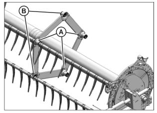
Figure 5.170: Tine Tube Supports
