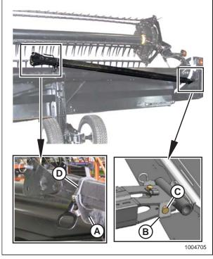
Figure 3.108: Tow-Bar Removal – Right Side
