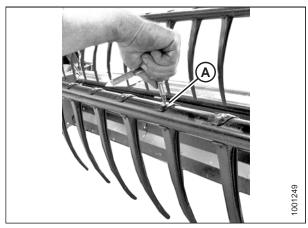
Figure 5.164: Installing Finger
