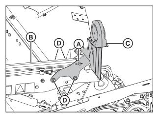
Figure 3.37: Left Reel Arm Cylinder in Aft Position
