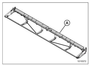
Figure 6.15: D1 Series Backsheet Extensions
