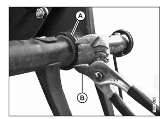
Figure 5.194: Clamp on Bushing
