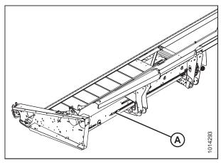
Figure 3.70: Chain Adjustment Bolt – Left Shown, Right Similar
