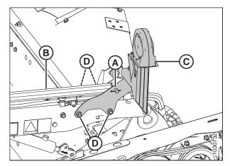
Figure 3.43: Left Reel Arm Cylinder in Aft Position
