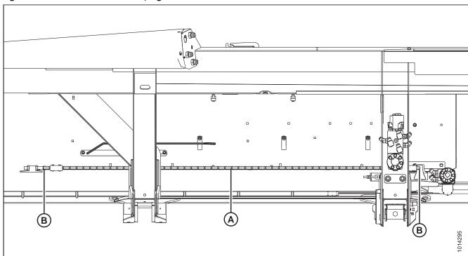
4. Measure to ensure chain midpoint (A) is 25–50 mm (1–2 in.) lower than the chain ends (B).
