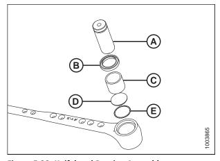
Figure 5.28: Knifehead Bearing Assembly
