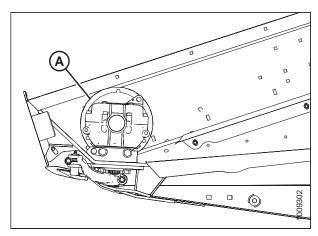
Figure 3.31: Knife Drive Pulley
