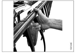
Figure 5.163: Installing Finger
