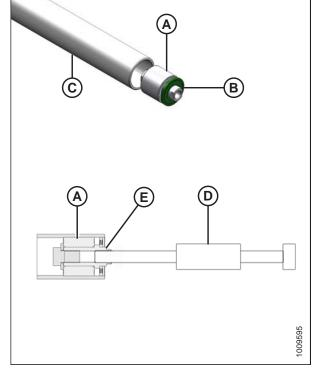
Figure 5.124: Idler Roller Bearing
