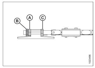
Figure 3.71: Chain Adjustment Bolt – Left Shown, Right Similar
