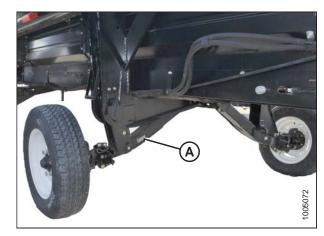
Figure 2: Slow Speed Transport / Stabilizer Wheel
