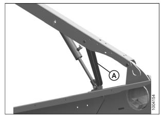
Figure 3.5: Reel Safety Prop - Left Outer Arm
