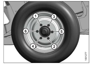
Figure 5.234: Bolt Tightening Sequence
