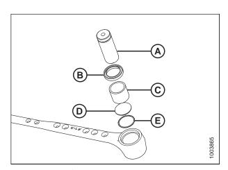
Figure 5.29: Knifehead Bearing Assembly
