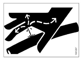
Figure 1.12: Hydraulic Pressure Hazard
