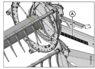
Figure 5.154: Fore-Aft Position Decal
