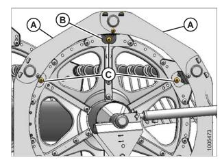
Figure 5.202: Reel Endshield Supports
