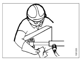
Figure 1.11: Testing for Hydraulic Leaks
