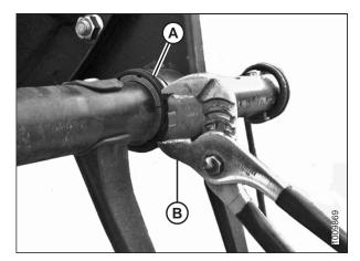
Figure 5.188: Clamp on Bushing
