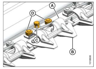
Figure 5.49: Stub Guard Sheet Metal Hold-Down
