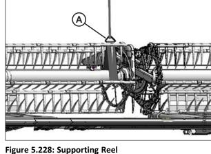
4. Remove four bolts (A) securing the reel tube to U-joint flange (B).
