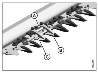
Figure 5.45: Double Knife Center Guard Hold-Down
