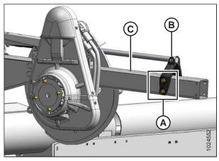
Figure 3.39: Center Arm - Aft Position
