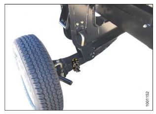
Figure 3.104: Left Wheel in Transport Position
