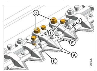
Figure 5.48: Double-Knife Center Stub Guard
