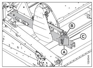
Figure 3.35: Right Reel Arm Cylinder in Aft Position
