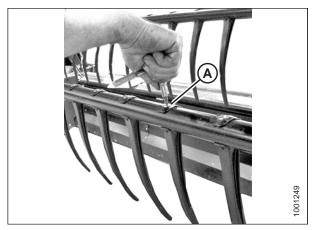
Figure 5.161: Removing Plastic Fingers
