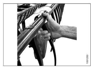
Figure 5.162: Removing Plastic Fingers
