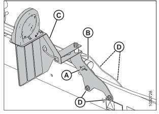
Figure 3.42: Left Reel Arm Cylinder in Forward Position
