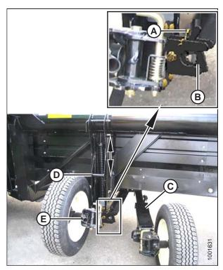
Figure 3.102: Separating Axles
