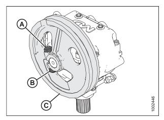
Figure 5.58: Knife Drive Box and Pulley
