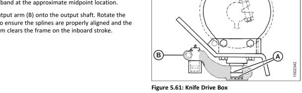
6. Position output arm (A) to the farthest outboard position. Move output arm (A) up or down on the splined shaft until it is almost contacting knifehead (B) (exact clearance [C] is set during the knifehead pin installation).
