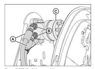
Figure 5.227: Reel Motor and Hoses
