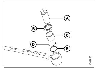
Figure 5.28: Knifehead Bearing Assembly
