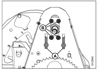
Figure 5.224: Reel Drive Motor Mounting Holes
