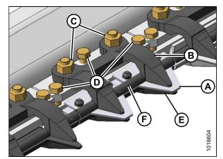
Figure 5.47: Normal Stub Guard Forged Hold-Down
