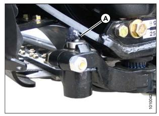
Figure 5.6: Every 25 Hours A - Knifehead (Single Knife [1 Place]; Double Knife [2 Places])
