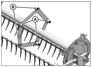
Figure 5.169: Tine Tube Supports
