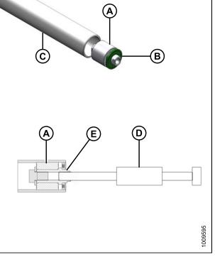
Figure 5.124: Idler Roller Bearing
