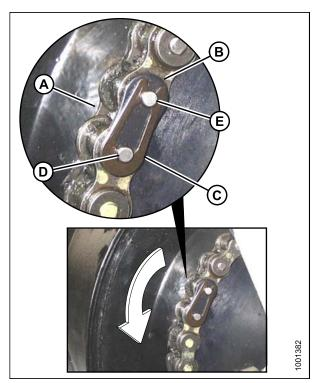
Figure 5.1: Chain Link Connector
