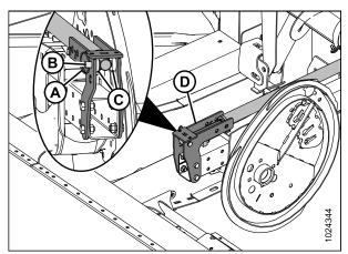
Figure 3.46: Center Reel Arm in Forward Position
