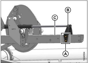
Figure 3.41: Right Reel Arm Cylinder in Aft Position
