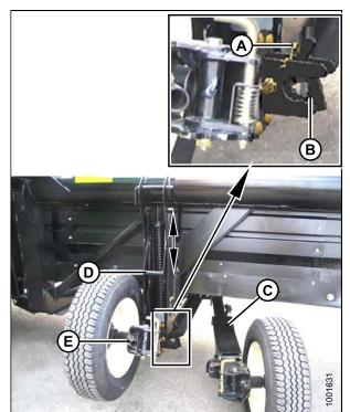
Figure 3.101: Separating Axles
