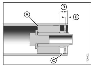
Figure 5.132: Idler Roller Bearing
