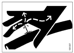
Figure 1.12: Hydraulic Pressure Hazard
