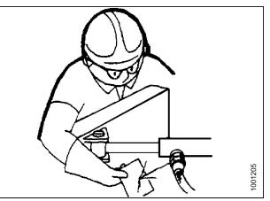
Figure 5.4: Testing for Hydraulic Leaks
