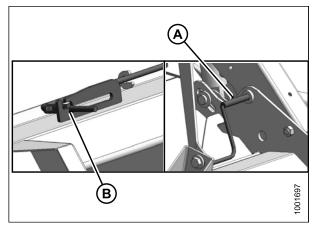
Figure 3.6: Reel Safety Prop – Center Arm
