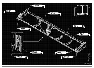
Figure 5.13: Double-Knife Header Master Grease Point Decal
