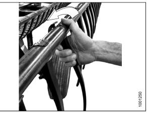
Figure 5.161: Removing Plastic Fingers
