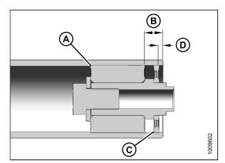
Figure 5.125: Idler Roller Bearing
