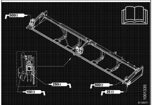
Figure 5.12: Single-Knife Header Master Grease Point Decal
