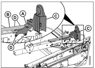
Figure 3.37: Left Reel Arm Cylinder in Aft Position
