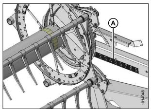
Figure 5.154: Fore-Aft Position Decal
