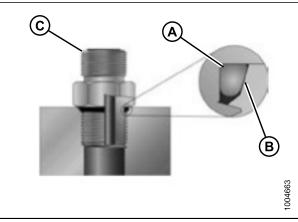
Figure 8.8: Hydraulic Fitting
