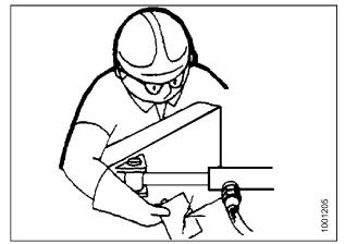
Figure 1.11: Testing for Hydraulic Leaks
