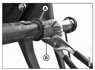
Figure 5.193: Clamp on Bushing
