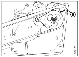
Figure 5.68: Single and Non-Timed Double-Knife Drive
