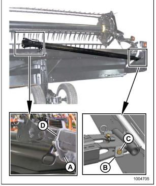
Figure 3.107: Tow-Bar Removal – Right Side
