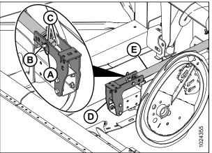
Figure 3.47: Center Reel Arm in Aft Position
