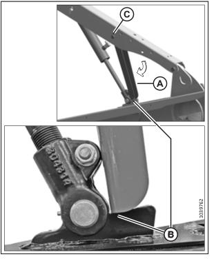
Figure 3.3: Engaged Reel Safety Prop – Left Shown
