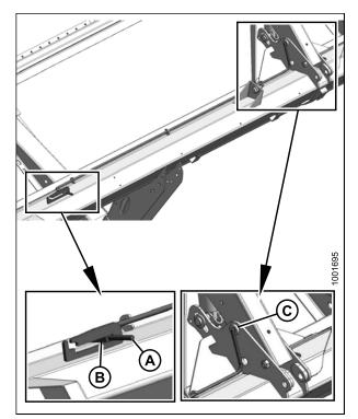
Figure 3.4: Reel Safety Prop – Center Arm
