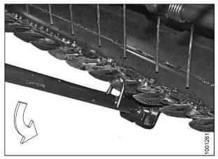
Figure 5.34: Downward Adjustment
