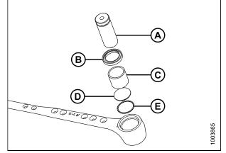
Figure 5.29: Knifehead Bearing Assembly
