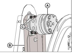
Figure 5.225: Reel Drive Motor
