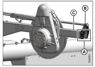
Figure 3.38: Center Arm – Forward Position
