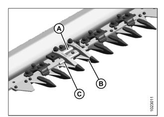
Figure 5.45: Double Knife Center Guard Hold-Down
