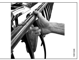
Figure 5.162: Installing Finger
