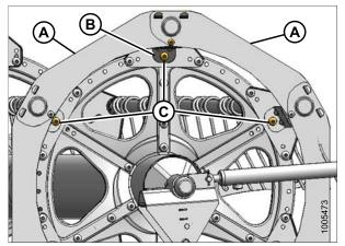
Figure 5.201: Reel Endshield Supports
