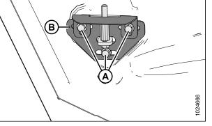
Figure 3.16: Left Endshield Latch Assembly
