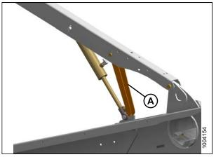
Figure 3.5: Reel Safety Prop – Left Side Outer Arm
