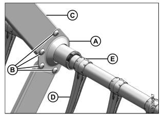
Figure 5.173: Tine Tube Support
