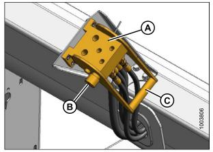
Figure 4.6: Reel Hydraulics Receptacle
