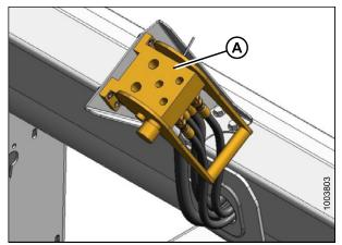
Figure 4.9: Closed Receptacle Cover
