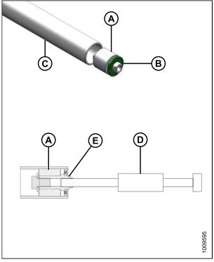
Figure 5.131: Idler Roller Bearing
