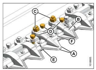
Figure 5.48: Double-Knife Center Stub Guard
