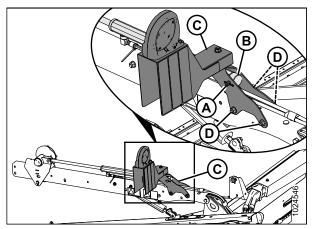
Figure 3.36: Left Reel Arm Cylinder in Forward Position
