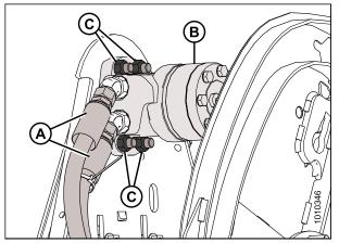
Figure 5.223: Reel Motor and Hoses
