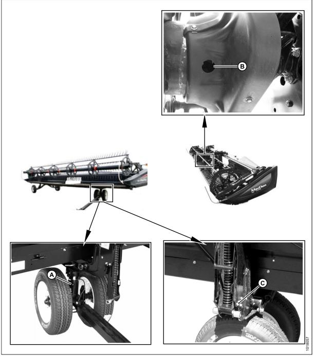
A - Front Wheel Pivot (1 Place) C - Frame/Wheel Pivot (1 Place) - Both Sides
