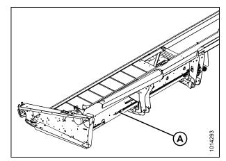
Figure 3.70: Chain Adjustment Bolt – Left Shown, Right Similar
