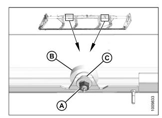
Figure 5.96: Cross-Shaft Support
