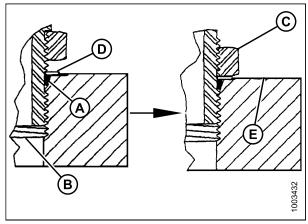
Figure 8.7: Hydraulic Fitting
