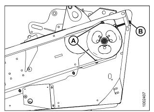
Figure 5.53: Single and Non-Timed Double-Knife Drive
