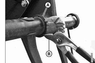
Figure 5.181: Clamp on Bushing
