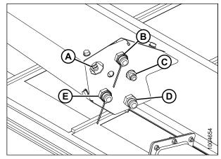
Figure 4.3: Header Receptacles A - Electrical Connector C - Case Drain (Double Knife) E - Return
