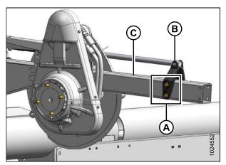
Figure 3.39: Center Arm – Aft Position
