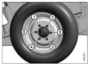
Figure 5.233: Bolt Tightening Sequence
