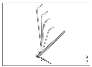
Figure 6.20: Swath Forming Rods
