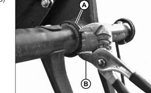
Figure 5.187: Clamp on Bushing
