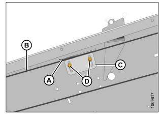
Figure 5.87: Left Side Belt Guide
