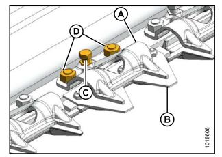
Figure 5.49: Stub Guard Sheet Metal Hold-Down
