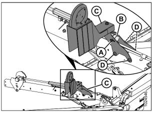
Figure 3.42: Left Reel Arm Cylinder in Forward Position
