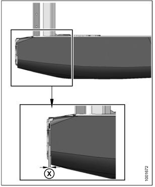
Figure 3.14: Gap between Endshield and Header Frame
