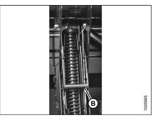
Figure 3.99: Locking Linkage
