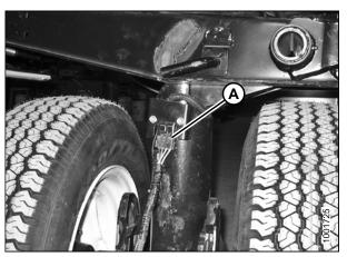
Figure 3.85: Wiring Connector
