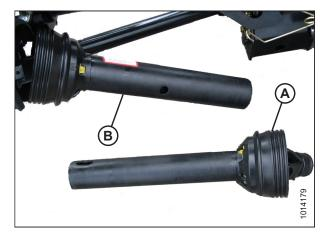
Figure 5.41: Separated Driveline
