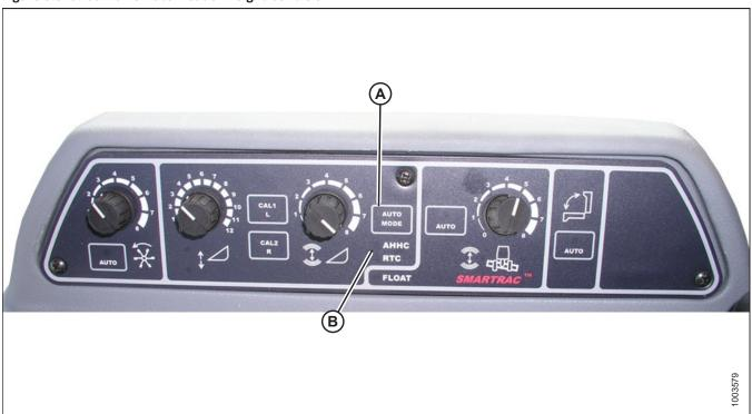
1. Press AUTO MODE button (A) until AHHC LED light (B) begins flashing. If the RTC light is flashing, press AUTO MODE button (A) again until it switches to AHHC.
