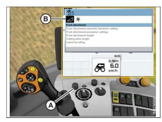
Figure 3.333: CLAAS Combine Display, Console, and Control Handle
