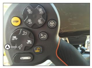
Figure 3.411: Header Down Switch
