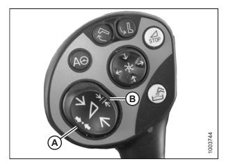
**Figure 3.319: Control Handle Buttons**
