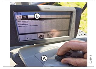
Figure 3.347: CLAAS Combine Display and Console
