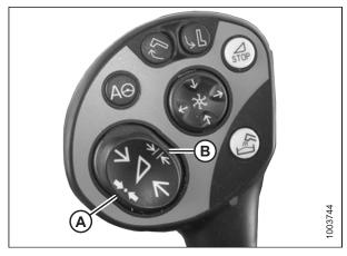
Figure 3.327: CLAAS Control Handle Buttons
