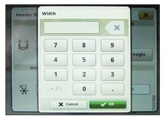
Figure 3.501: John Deere S7 Display – Setting Header Width
