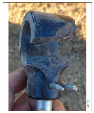
Figure 5.77: Broken Finger Holder
