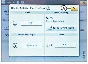
Figure 3.502: John Deere S7 Display – Header Details Window
