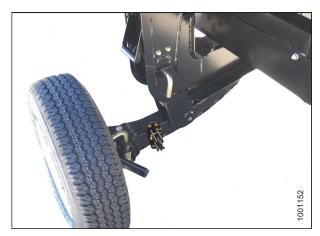
Figure 3.607: Left Wheel in Transport Position
