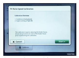
Figure 3.518: John Deere S7 Display – Feeder House Calibration
