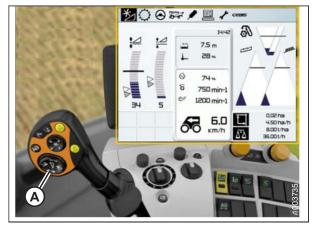
Figure 3.338: CLAAS Combine Display, Console, and **Control Handle**
