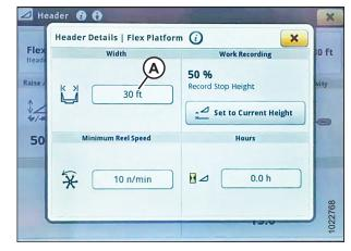
Figure 3.500: John Deere S7 Display – Header Details Window
