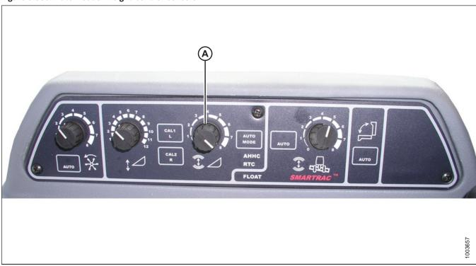
SENSITIVITY ADJUSTMENT dial (A) controls the distance the cutterbar must travel up or down before the auto header height control (AHHC) reacts and raises or lowers the feeder house.
