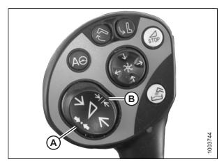
Figure 3.331: CLAAS Control Handle Buttons
