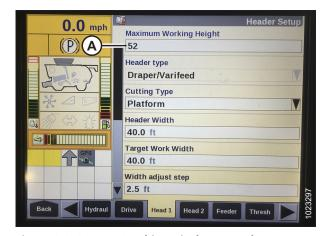
Figure 3.253: Case Combine Display – Header Setup Page
