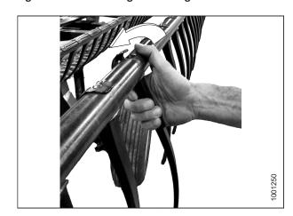
Figure 5.280: Removing Plastic Finger
