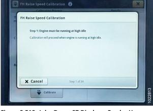
Figure 3.519: John Deere S7 Display – Feeder House Calibration
