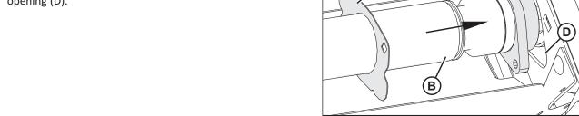
4. Slide left end of drive roller (A) onto motor spline (B) as shown.
