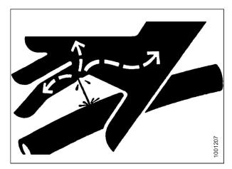
Figure 1.12: Hydraulic Pressure Hazard
