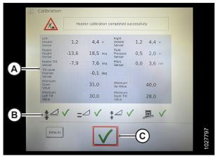
Figure 3.220: Completed Calibration Page
