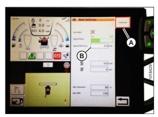
Figure 3.400: Reel Settings Calibration
