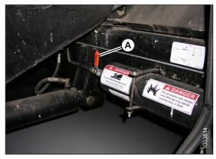
Figure 3.382: Combine Accumulator ON/OFF Switch A - Accumulator Lever (Off Position)
