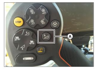
Figure 3.224: AHHC on Control Handle
