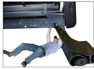
Figure 5.224: Installing Draper
