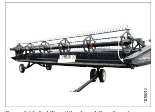
Figure 6.16: Stabilizer Wheels and Slow Speed Transport
