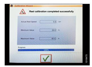
Figure 3.403: Calibration Progress
