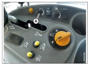
Figure 3.306: Height Adjustment Knob on the Combine Control Console
