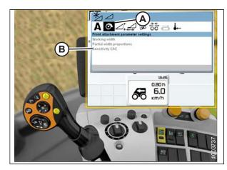
Figure 3.340: CLAAS Combine Display, Console, and Control Handle
