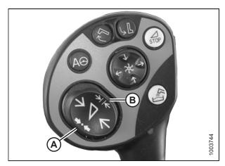
Figure 3.317: Control Handle Buttons
