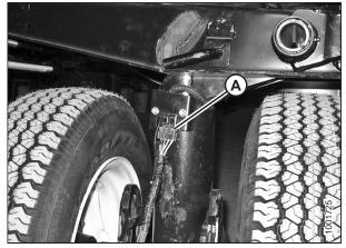
Figure 3.588: Wiring Connector
