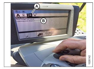
Figure 3.348: CLAAS Combine Display and Console
