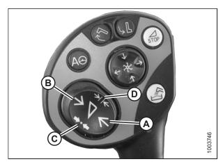
Figure 3.320: Control Handle Buttons
