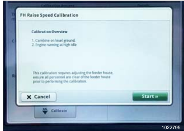
Figure 3.403: John Deere S7 Display – Feeder House Calibration
