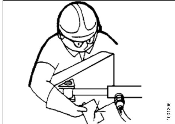
Figure 1.11: Testing for Hydraulic Leaks
