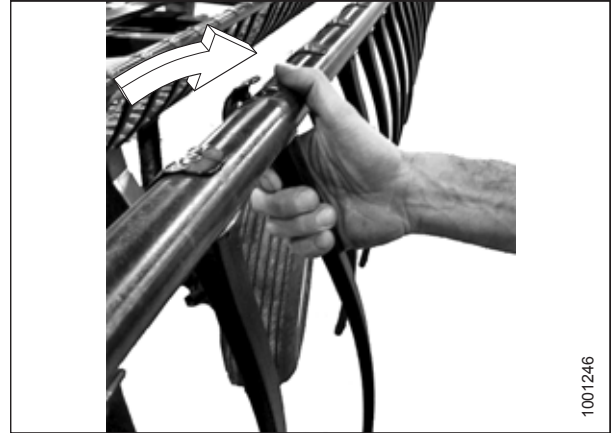
Figure 5.252: Installing Plastic Finger
