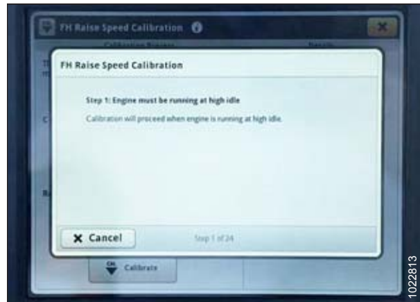
Figure 3.404: John Deere S7 Display – Feeder House Calibration
