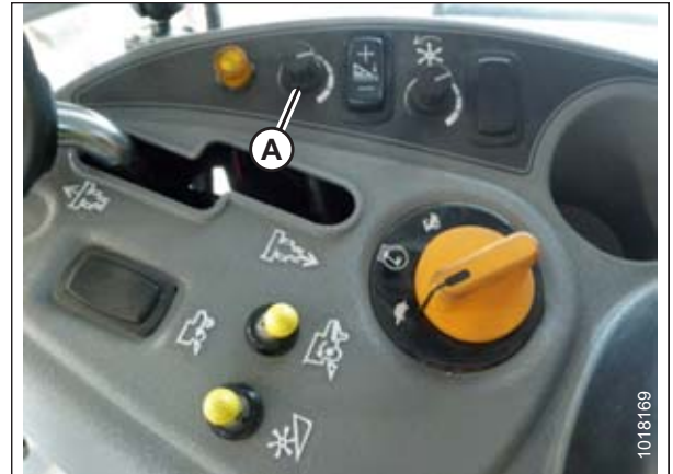
Figure 3.260: Height Adjustment Knob on the Combine Control Console
