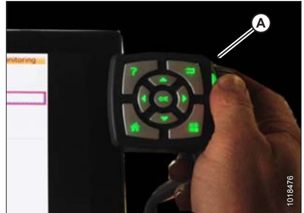
Figure 3.311: Adjustment Wheel on Right Side of Tyton Terminal
