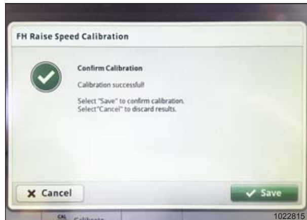
Figure 3.405: John Deere S7 Display – Feeder House Calibration
