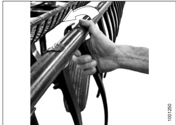
Figure 5.251: Removing Plastic Finger
