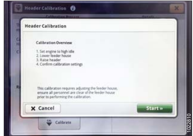
Figure 3.411: John Deere S7 Display – Header Calibration
