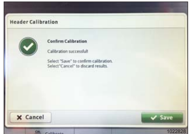
Figure 3.412: John Deere S7 Display – Header Calibration
