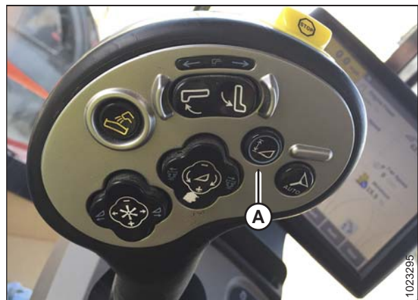
Figure 3.241: Case Combine Control Handle
