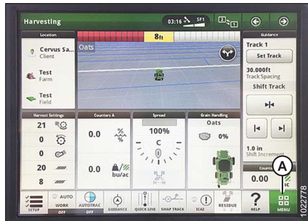
Figure 3.489: John Deere S7 Display – Harvesting Page
