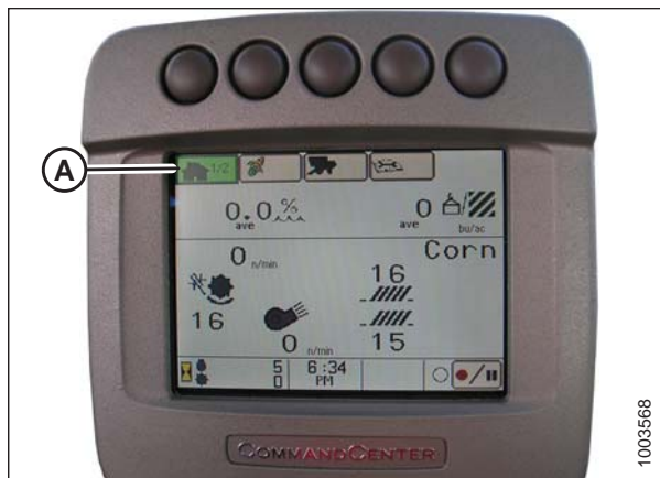
Figure 3.406: John Deere Combine Display
