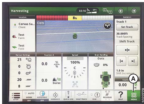
Figure 3.482: John Deere S7 Display – Harvesting Page
