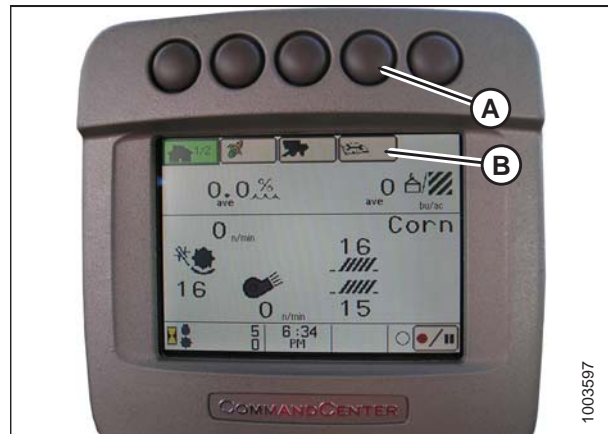
Figure 3.412: John Deere Combine Display
