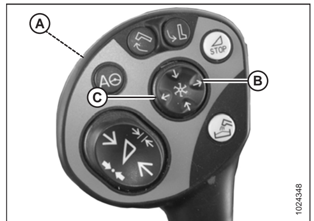
Figure 3.87: CLAAS 500 Control Handle
