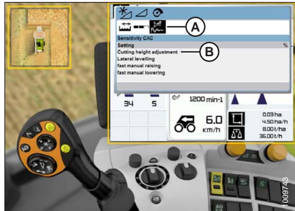
Figure 3.330: CLAAS Combine Display
