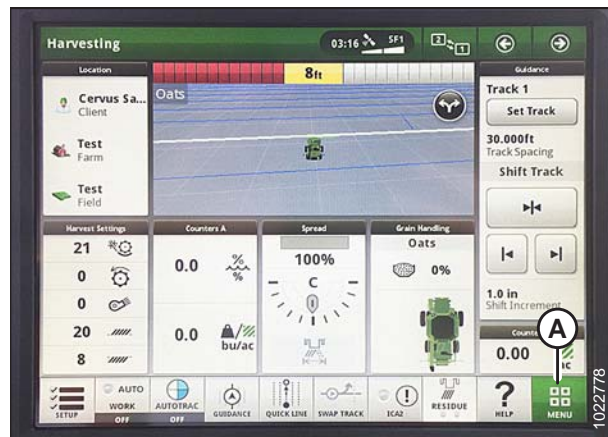
Figure 3.478: John Deere S7 Display – Harvesting Page
