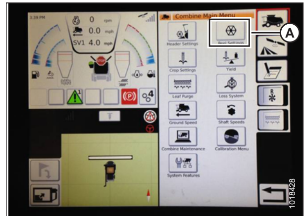
Figure 3.367: Reel Settings on Combine Main Menu
