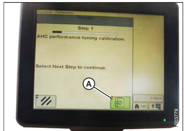
Figure 3.433: John Deere Combine Display
