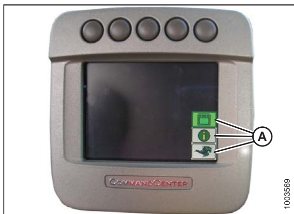
Figure 3.407: John Deere Combine Display
