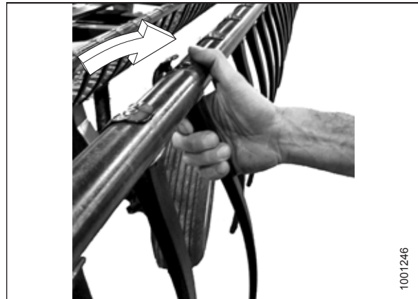
Figure 5.256: Installing Plastic Finger
