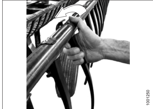
Figure 5.255: Removing Plastic Finger
